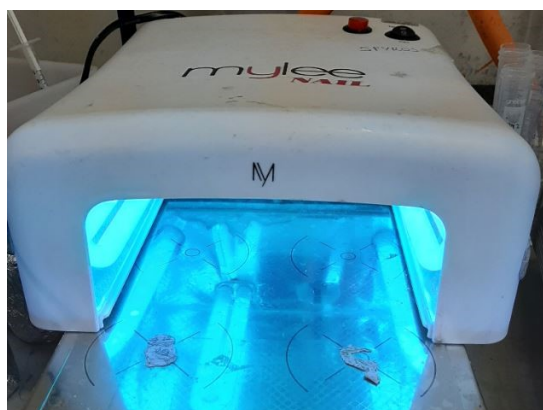
Figure S1. UV curing lamp equipped with four 9 W bulbs emitting at \lambda_{\text{max}} \sim 365 nm for small scale
