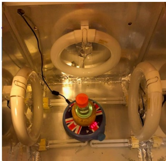
Figure S2. Custom-made UV box set up with \lambda_{\text{max}} \sim 360 nm used for higher scale photo polymerisations.
