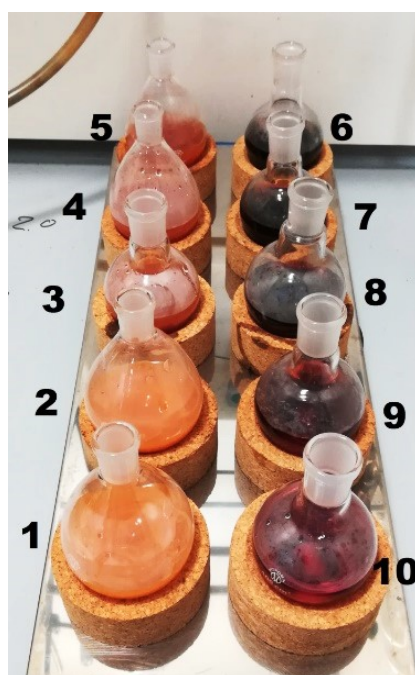
Figure S6. Experiment with different equivalents of \text{NaIO}_4 . The left row corresponds to poly(dopaazide) and the right row presents PDA. Flask number: 1 and 10 (0.1 eq. \text{NaIO}_4 ), 2 and 9 (0.2 eq. \text{NaIO}_4 ), 3 and 8 (0.5 eq. \text{NaIO}_4 ), 4 and 6 (1.0 eq. \text{NaIO}_4 ), 5 and 6 (2.0 eq. \text{NaIO}_4 )
