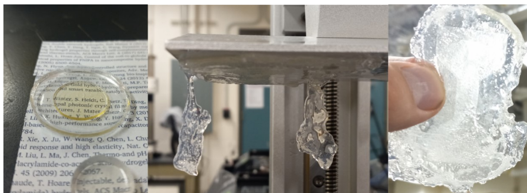
SI Figure 12. Curing and 3D printing of BMAP/PS80-SH resins. As shown on the left, the resins were transparent and stiff when cured in plates under UV light. However, the resin completely gelled / cured during printing as shown in the middle. On the right, the faint outline of the intended print (dogbone) could be seen under light embedded in a gel-like matrix.
