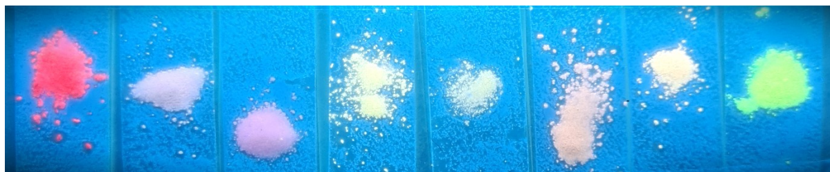
Figure S27: Digital photographs of UCY-15 (RE) under a conventional UV lamp operating at 365nm. From left to right: UCY-15 (Eu), UCY-15 (Y 90 Eu 5 Tb 5 ), UCY-15 (Y 87.5 Eu 5 Tb 7.5 ), UCY-15 (Y 85 Eu 5 Tb 10 ), UCY-15 (Y 87.5 Eu 7.5 Tb 5 ), UCY-15 (Y 85 Eu 10 Tb 5 ), UCY-15 (Y 85 Eu 7.5 Tb 7.5 ) and UCY-15 (Tb).
