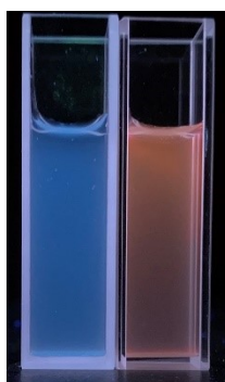
Fig. S20. Photographs of L@Mg-Al-Eu-LDHs with and without DPA under 254 nm UV light.
