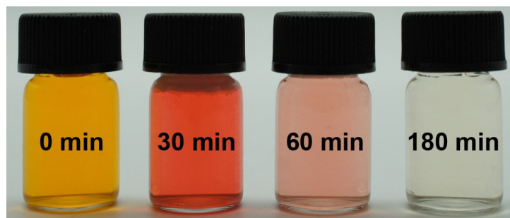
Figure S7. Time-dependent digital photographs of MO aqueous solution treated by Pt-ZIS micromotors at the best condition (8-Pt-ZIS||H 2 O 2 +Vis). The color change from orange to red is due to the addition of H 2 O 2 .
