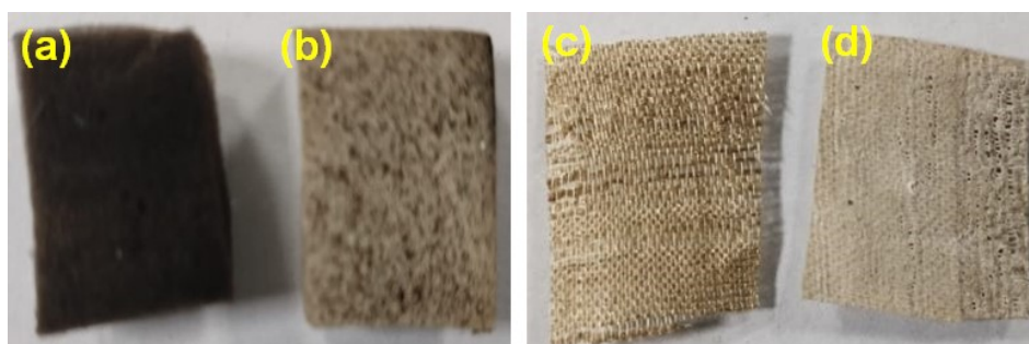
Fig. S16. Digital images of (a) polymer-coated sponge, (b) SH-UiO-66' @sponge composite, (c) polymer-coated silk membrane and (d) SH-UiO-66' @silk membrane.
