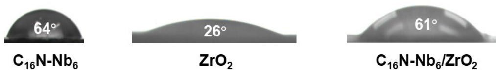
Figure S6. Images of water contact angles of C_{16}N-Nb_6 , ZrO_2 and C_{16}N-Nb_6/ZrO_2 .
