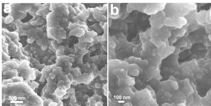
**Fig. S1** Low-magnification (a) and high-magnification (b) SEM images of the SnO<sub>2</sub> NSs/HGF electrodes after charge/discharge cycles.
