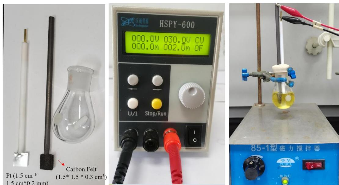
**Figure S1.** Reaction set-up for milligram-scale electrolysis. The anode is carbon felt electrode ( $1.5\text{ cm} \times 1.5\text{ cm} \times 0.3\text{ cm}$ ) while the cathode is platinum electrode ( $1.5\text{ cm} \times 1.5\text{ cm} \times 0.2\text{ mm}$ ).
