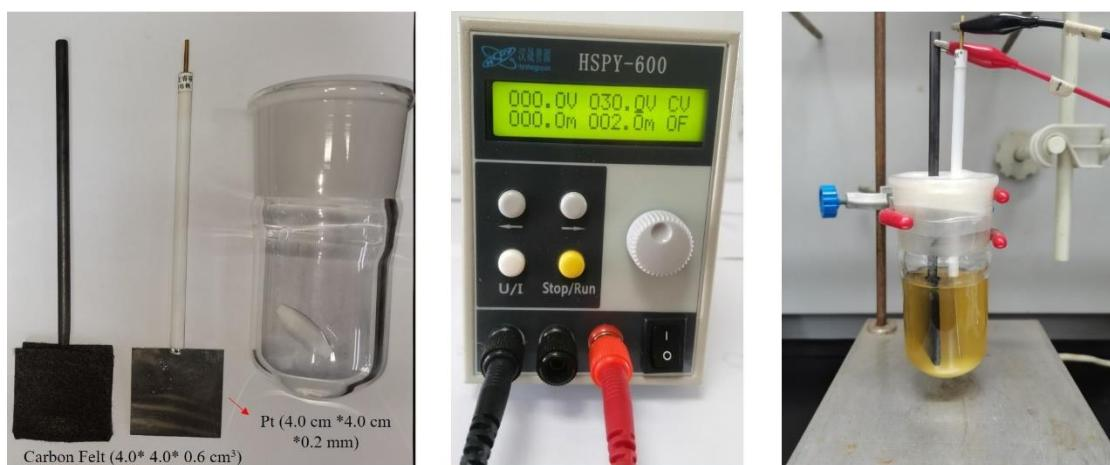
**Figure S2.** Reaction set-up for gram-scale electrolysis. The anode is carbon felt electrode ( $4.0\text{ cm} \times 4.0\text{ cm} \times 0.6\text{ cm}$ ) while the cathode is platinum electrode ( $4.0\text{ cm} \times 4.0\text{ cm} \times 0.2\text{ mm}$ ).
