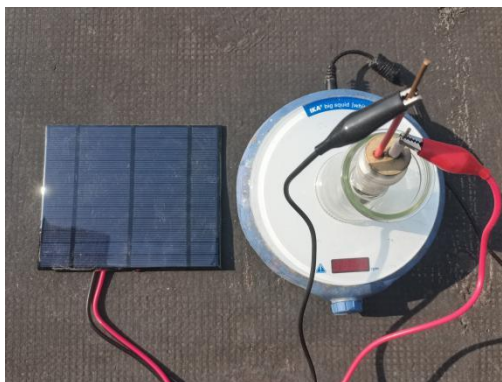
Figure S3 Electrolysis setup with solar cell (135 mm*165mm) as electricity supply (10:00-12:00 am, May 16 th , 2022 at Hefei, China)
