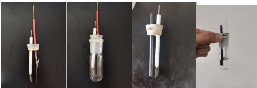
Figure S1 Electrolysis setup (graphite rod: diameter 0.6 cm, length 10 cm; lead plate: 1.5 cm (width) *1.5 cm (immersion depth); platinum plate: 1.5 cm *1.5 cm)
