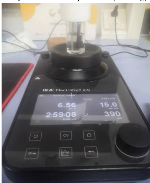
Figure S5. Electrolysis using IKA ElectraSyn 2.0.
