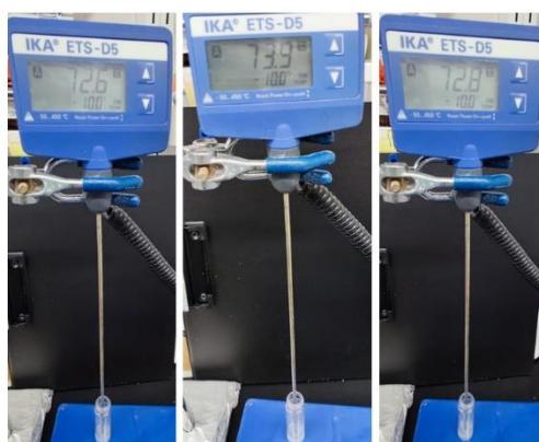
Fig. S10 Temperature measured after heating the mixture of G1 , G2 and DMS with a heat gun for 30 seconds. The test was repeated for 3 times.
