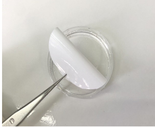
Fig.S4 Digital photo of membrane (M2) after immersing into 2000 ppm \text{Na}_2\text{SO}_4 solution for 24h
