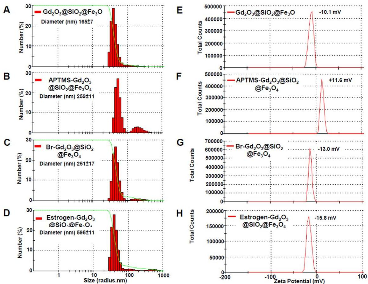
**Figure S4:** A-D- Dynamic light scattering of the nanocarriers (cube shaped iron oxide as a core) in water showed an increase in average hydrodynamic diameter of nanocarriers after different conjugation steps. E-H- Zeta potential measurements displayed a change in surface charge after the attachment of different molecule used for the conjugation of estrogen molecules.
