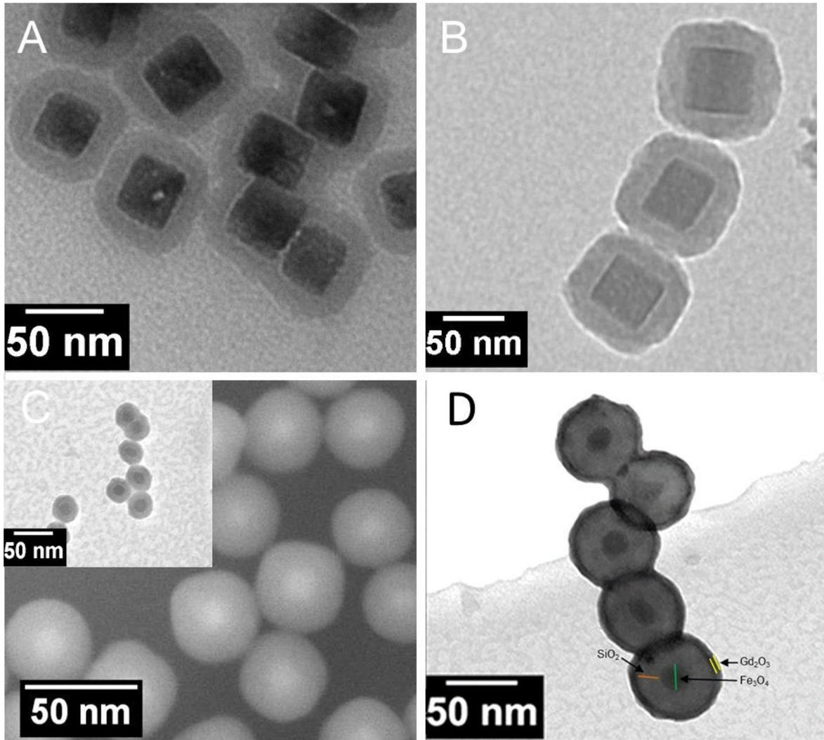
**Figure S2:** A-B: TEM images with different magnification of SiO<sub>2</sub>@Fe<sub>3</sub>O<sub>4</sub>(cubes) NPs, C- SEM image of SiO<sub>2</sub>@Fe<sub>3</sub>O<sub>4</sub>(spheres) NPs, and D- TEM image of Gd<sub>2</sub>O<sub>3</sub>@SiO<sub>2</sub>@Fe<sub>3</sub>O<sub>4</sub>(spheres) showing the clear demarcation of thin layer of gadolinium oxide ( $15 \pm 5$  nm) on core shell structure.
