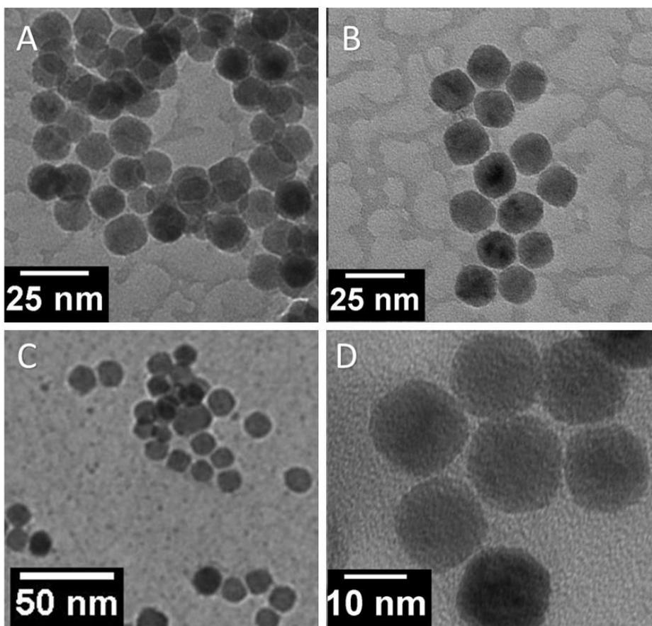
**Figure S1:** TEM images of iron oxide particles with different magnification **A-B** oleic acid-capped Fe<sub>3</sub>O<sub>4</sub> nanospheres, **C-D** Fe<sub>3</sub>O<sub>4</sub> NPs after the removal of oleic acid
