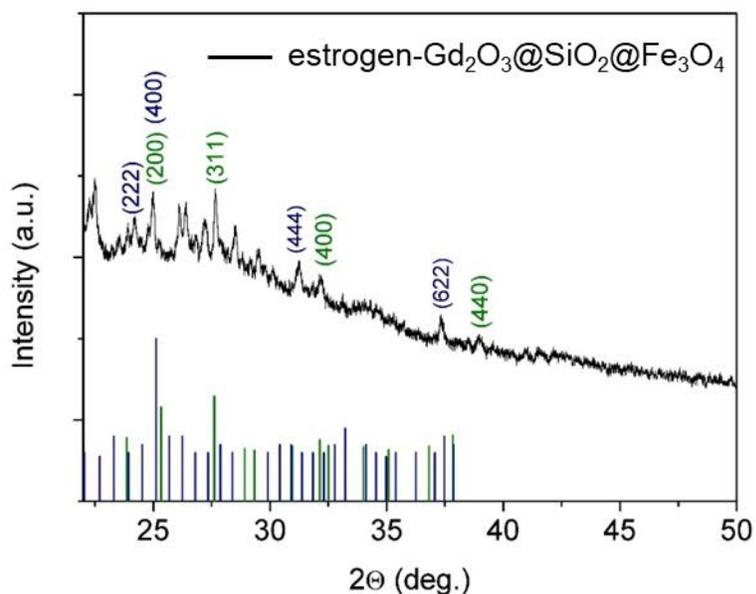
**Figure S5:** XRD diffraction pattern of Gd<sub>2</sub>O<sub>3</sub>@SiO<sub>2</sub>@Fe<sub>3</sub>O<sub>4</sub> NPs after conjugation of estrogen via click reaction. The references for magnetite (JCPDS C72-2303) is in green, and for Gd<sub>2</sub>O<sub>3</sub> (JCPDS C12-0797) in blue.
