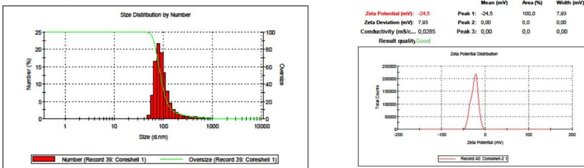
**Figure S8:** Dynamic light scattering of the nanocarriers (spherical iron oxide as a core) in water showed an increase in average hydrodynamic diameter of nanocarriers as compared to TEM analysis. Zeta potential measurements displayed a negative charge when no surface linker or ligand is attached.
