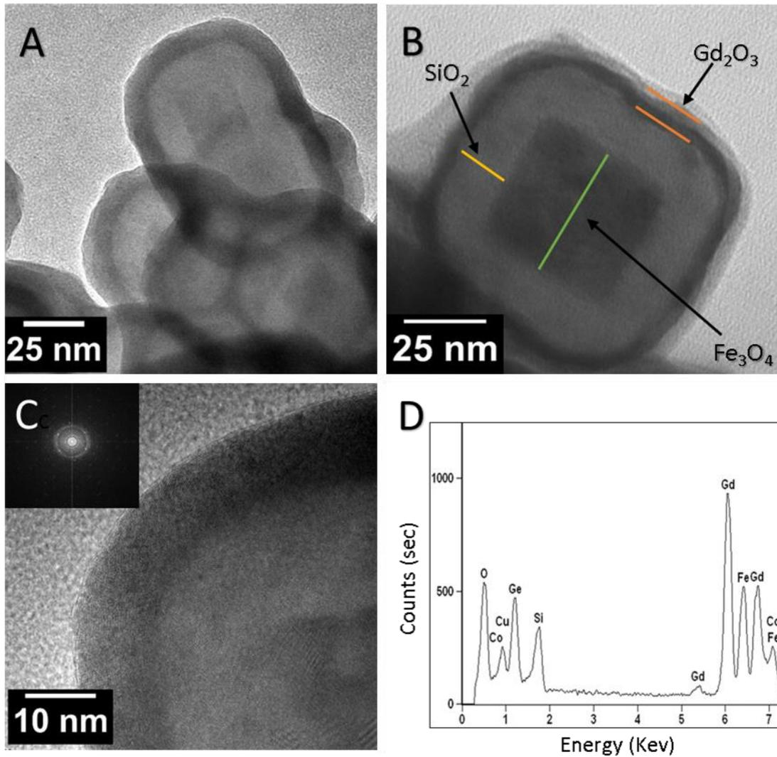
**Figure S3:** A-B- TEM Images of  $Gd_2O_3@SiO_2@Fe_3O_4(cubes)$  nanocarriers C- High resolution TEM of  $Gd_2O_3@SiO_2@Fe_3O_4(cubes)$  carriers (the inset for SAED pattern), and D- EDX analysis of  $Gd_2O_3@SiO_2@Fe_3O_4(cubes)$  nanocarriers
