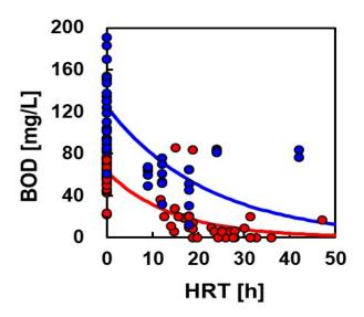
Supplemental Figure S1. Comparison of BOD removal by MFCs with and without partial aeration.
