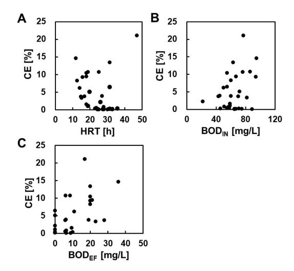
Supplemental Figure S2. Relationships between CE and the three parameters: HRT (A), BODIN (B), and BODEF (C).
