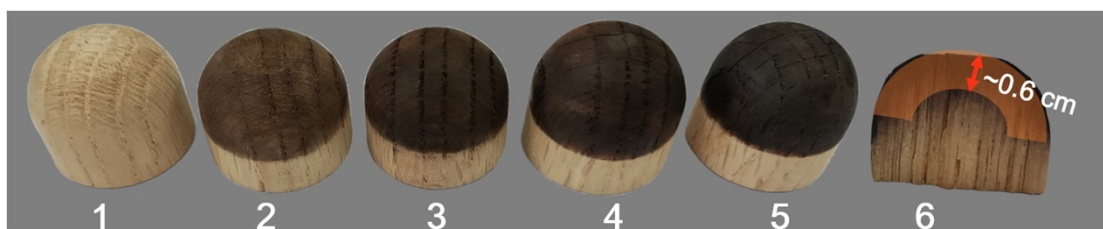
Figure S1. (1) Natural wood blocks with one semi-spherical end treated at 400 °C with different times (2-5) 10, 20, 25, and 30 min to form wC-s-s, and (6) longitudinal section of w-C-s-s-25 to reveal the thickness of carbon layers.
