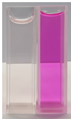
Figure S11. Optical image of RhB solution in seawater before and after irradiation of simulated light at 1 \text{ kW cm}^{-2} for 3 h in the presence of P25/wC-s-s-25.
