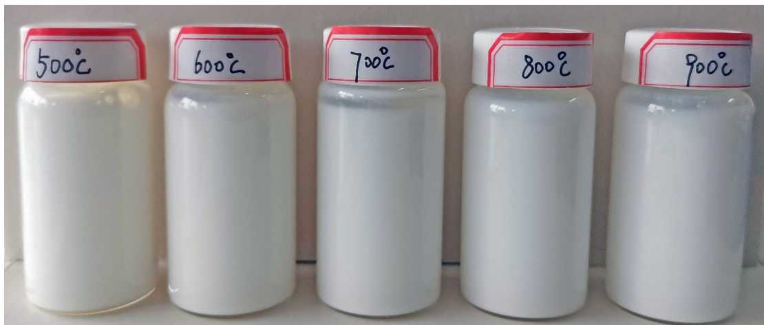
Fig. S5 Digital photo of polishing slurries prepared with the products calcined at 500, 600, 700, 800 and 900 °C (Sample A-E).
