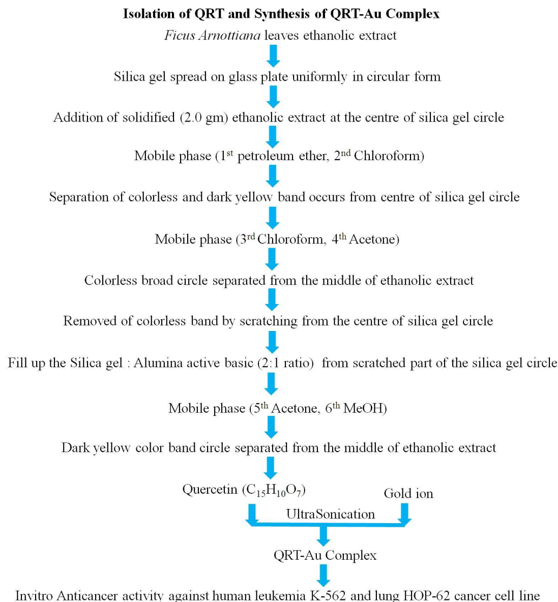
Fig. S1 Flow sheet diagram of isolation of QRT and synthesis of QRT-AuQDS.
