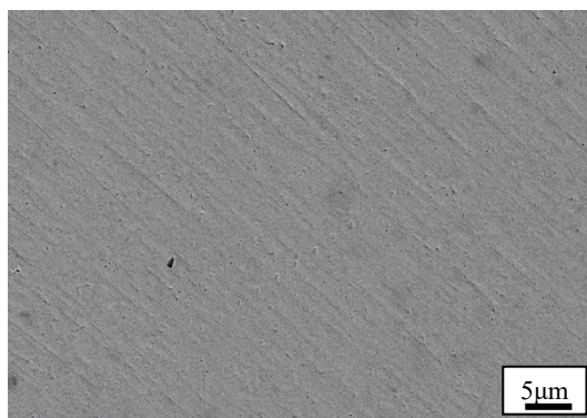
Fig.S3 SEM image of pure Au after CV test in 0.5 M KOH + 0.5 M CH 3 OH solution
