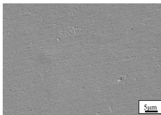
Fig.S6 SEM image of pure Au after CV test in 0.5 M H 2 SO 4 + 0.5 M HCOOH solution
