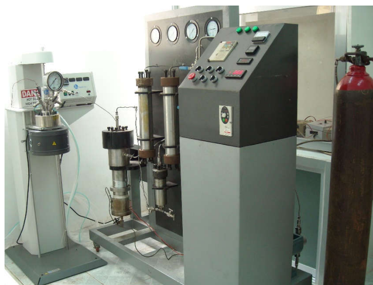
Figure S10. Supercritical CO 2 instrument made in Institute of Chemical Technology (ICT)-Vietnam Academy of Science and Technology (VAST) - Vietnam
