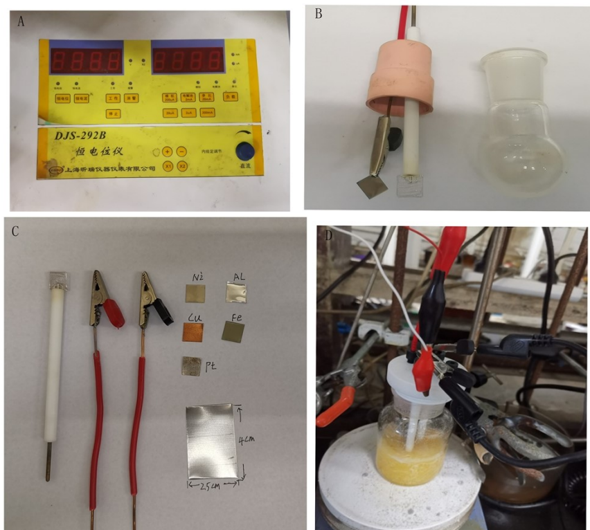
Figure S1. Electrolysis setup (A: Shanghai xirui DJS-292B constant potentiometer; B: Fe plate (1.0 * 1.0 cm 2 ), Pt net (1.0 * 10 cm 2 ), An undivided cell of 10 mL flask; C: Series of electrodes; D: Gram scale reaction device).
