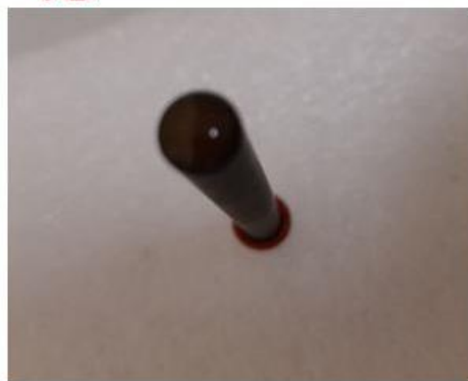
Figure S3. Photographs of (a) glassy carbon electrode, and (b) the CuO@S-doped g-C 3 N 4 nanocomposites modified glassy carbon electrode ( see the top side of the electrodes )
