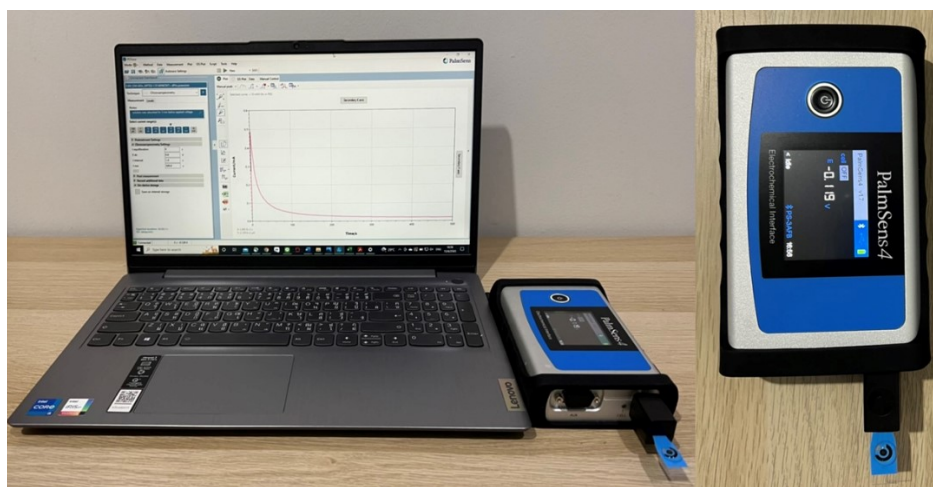
Fig. S7 Experimental setup of the portable enzymatic glucose sensor by chronoamperometric detection in glucose solution by PalmSens4 device connected with the modified electrode and linked to a laptop computer via Bluetooth or USB connector.
