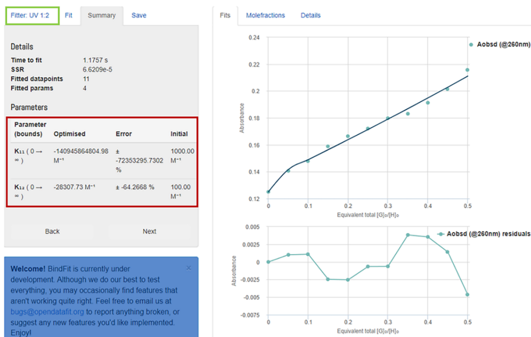
Fig. S4 Screenshot of the summary window of http://app.supramolecular.org/bindfit/ . This screenshot shows the raw data for the UV-Vis titration of BM with CT6 following the UV-Vis absorption values at 260 nm vs. the data fitted to the 1:2 UV binding model, the corresponding residual plot and the association constants with the calculated asymptotic standard errors.
