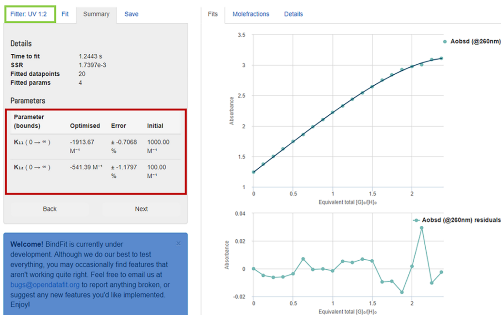
Fig. S7 Screenshot of the summary window of http://app.supramolecular.org/bindfit/ . This screenshot shows the raw data for the UV-Vis titration of the CT6/BM complex with AMP following the UV-Vis absorption values at 260 nm vs. the data fitted to the 1:2 UV binding model, the corresponding residual plot and the association constants with the calculated asymptotic standard errors.
