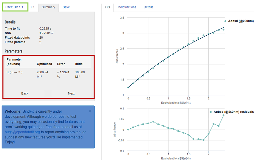
Fig. S6 Screenshot of the summary window of http://app.supramolecular.org/bindfit/ . This screenshot shows the raw data for the UV-Vis titration of the CT6/BM complex with AMP following the UV-Vis absorption values at 260 nm vs. the data fitted to the 1:1 UV binding model, the corresponding residual plot and the association constants with the calculated asymptotic standard errors.
