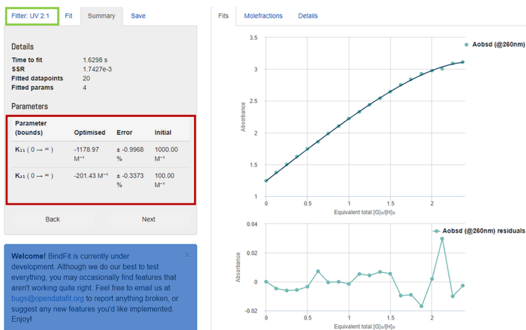
Fig. S8 Screenshot of the summary window of http://app.supramolecular.org/bindfit/ . This screenshot shows the raw data for the UV-Vis titration of the CT6/BM complex with AMP following the UV-Vis absorption values at 260 nm vs. the data fitted to the 2:1 UV binding model, the corresponding residual plot and the association constants with the calculated asymptotic standard errors.
