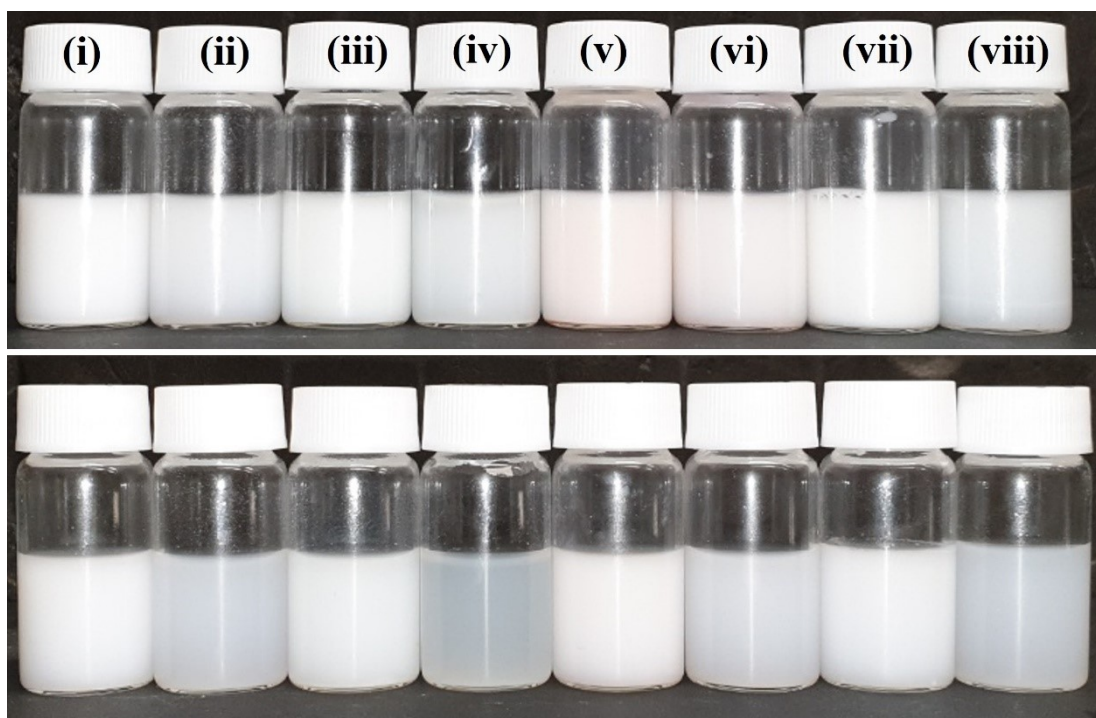
Figure S14. Whitening effect of the modified sunblock's with CNF at the high and low concentrations i.e., (i) oSB1 (50+), (ii) oSB1(50 + ) + 5g CNF, (iii) oSB2(50+), (iv) 2SB1(50 + ) + 5g CNF, (v) ioSB1(35+), (vi) ioSB1(35 + ) + 5g CNF, (vii) ioSB2(50 + ) and (viii) ioSB2(50 + ) + 5g CNF.
