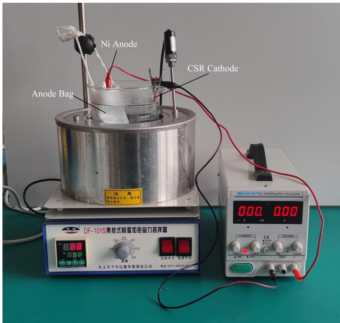
Fig. S1 An illustration of electroplating equipment used in the experiment (In order to clearly show the composition of the device, the liquid in the beaker was changed from electroplating solution to deionized water).
