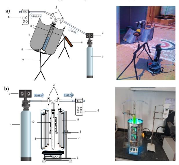
**Fig. (S1)** A schematic diagram of a) lab-scale UV-reactor; b) proto-type solar photobiogas reactors: 1-Nitrogen cylinder, 2- Gas pressure regulator, 3- Gas Faucet, 4-Reaction tube, 5- the magnetic stirrer, 6- Outgoing gas meter (CH<sub>4</sub>, H<sub>2</sub> detector), 7- Holder, 8-Reflective cylinder made of stainless steel, 9- Ultraviolet light bulbs, 10- Cooling fan and 11-Sun tracker stick.
