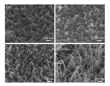
Fig. S1. The morphology of metal sulfides with different Ni/Co ratios (a) N51 sample (b) N42 sample (c) NC33 sample (d) NC15 sample
