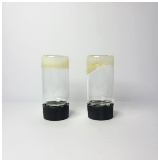
Fig. S2. Photographs of cured P(AMPSs/VIPS-co-AAm) hydrogel (left) and less cured P(AMPSs/VIPS) hydrogel (right).
