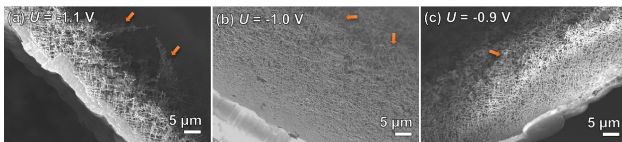
Figure S1. SEM images of cross-sections of Au nanowire network deposited at (a) U = -1.1 V, (b) U = -1.0 V (c) U = -0.9 V vs. Ag/AgCl.
