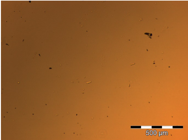
Figure S6 Microscopy images of cellulose acetate DS 0.17
