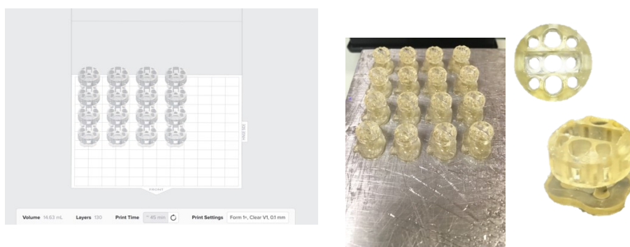
Supplementary Figure 2. Design on the FormLabs software, printed on the build plate and with support and removed support from the batch-based stirrer devices.
