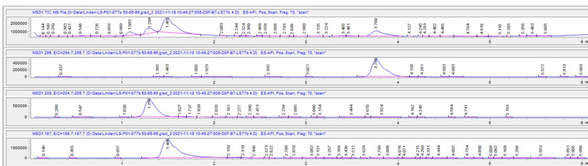
Figure S11: Separation and identification of mono-addition intermediate 3f and di-addition intermediate 5f using LC-MS while attempting to separate regioisomeric pyrazoles 4f and 4f' for the reaction of diketone 1f and phenyl hydrazine. The figure consists of the TIC from the mass spectrometer, followed by the EIC (extracted ion chromatogram) for the di-addition intermediate 5f ( m/z = 295.2 ), mono-addition intermediate 3f ( m/z = 205.2 ) and pyrazole products 4f/4f' ( m/z = 187.2 ).
