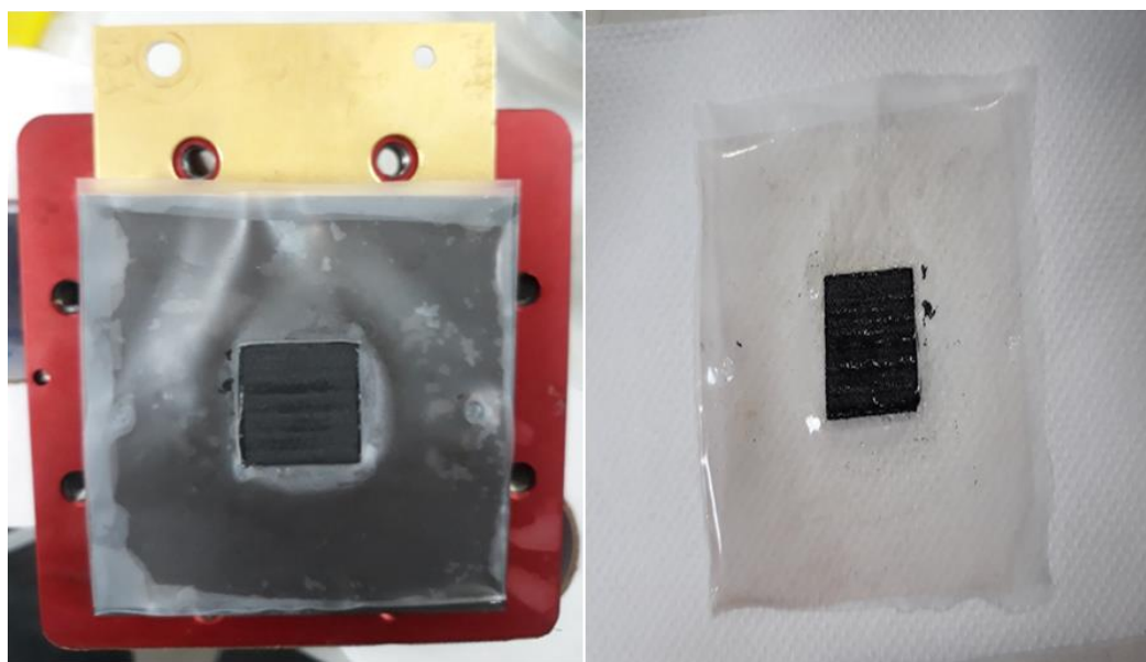
Fig.S12 a) Half-cell assembly of the fuel cell b) MEA after single cell testing
