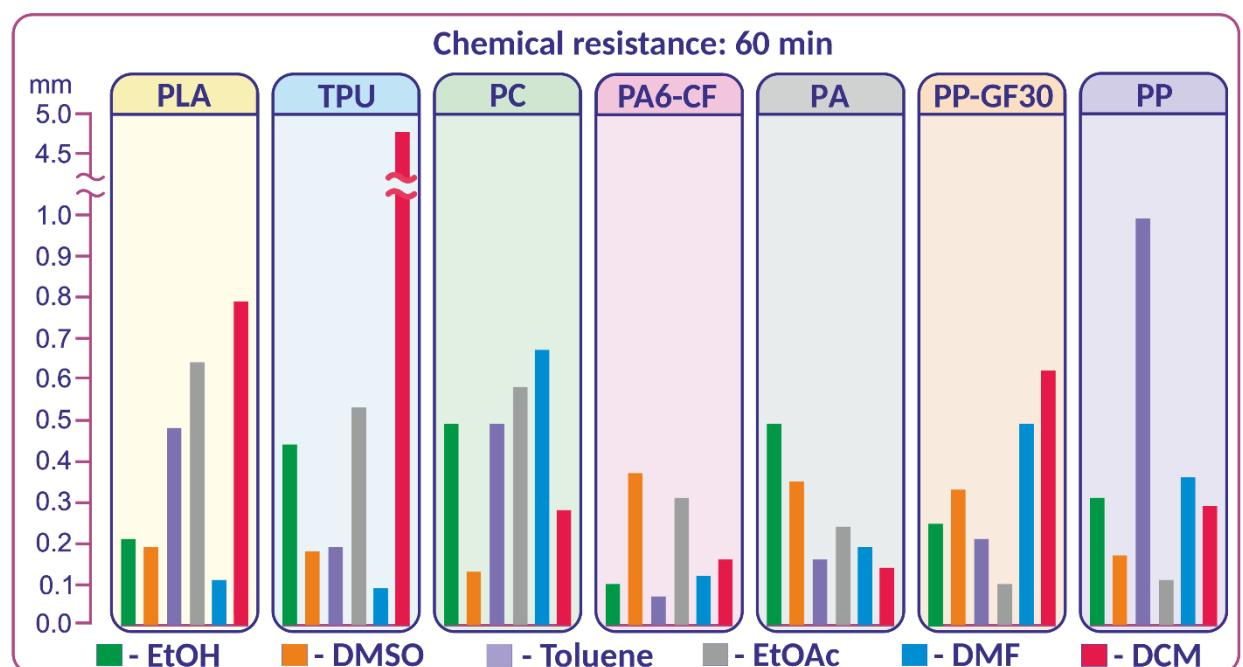
**Figure S20.** Diagram with quantitative calculations of the chemical resistance of 3D printed samples when exposed to various solvents for 60 minutes.
