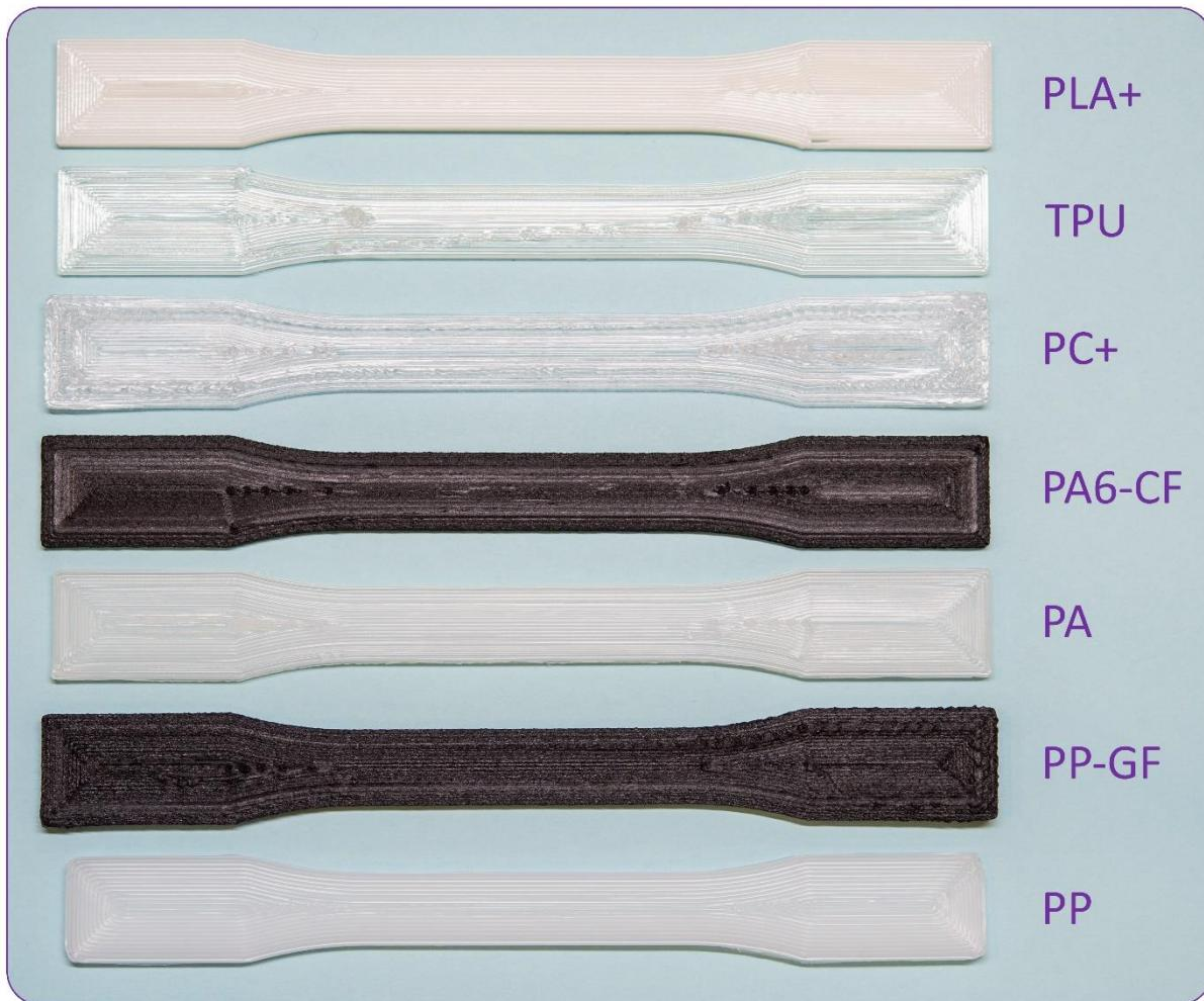
**Figure S32.** FFF samples for tensile testing with infill angle relative to the direction of load application equal to 0°.
