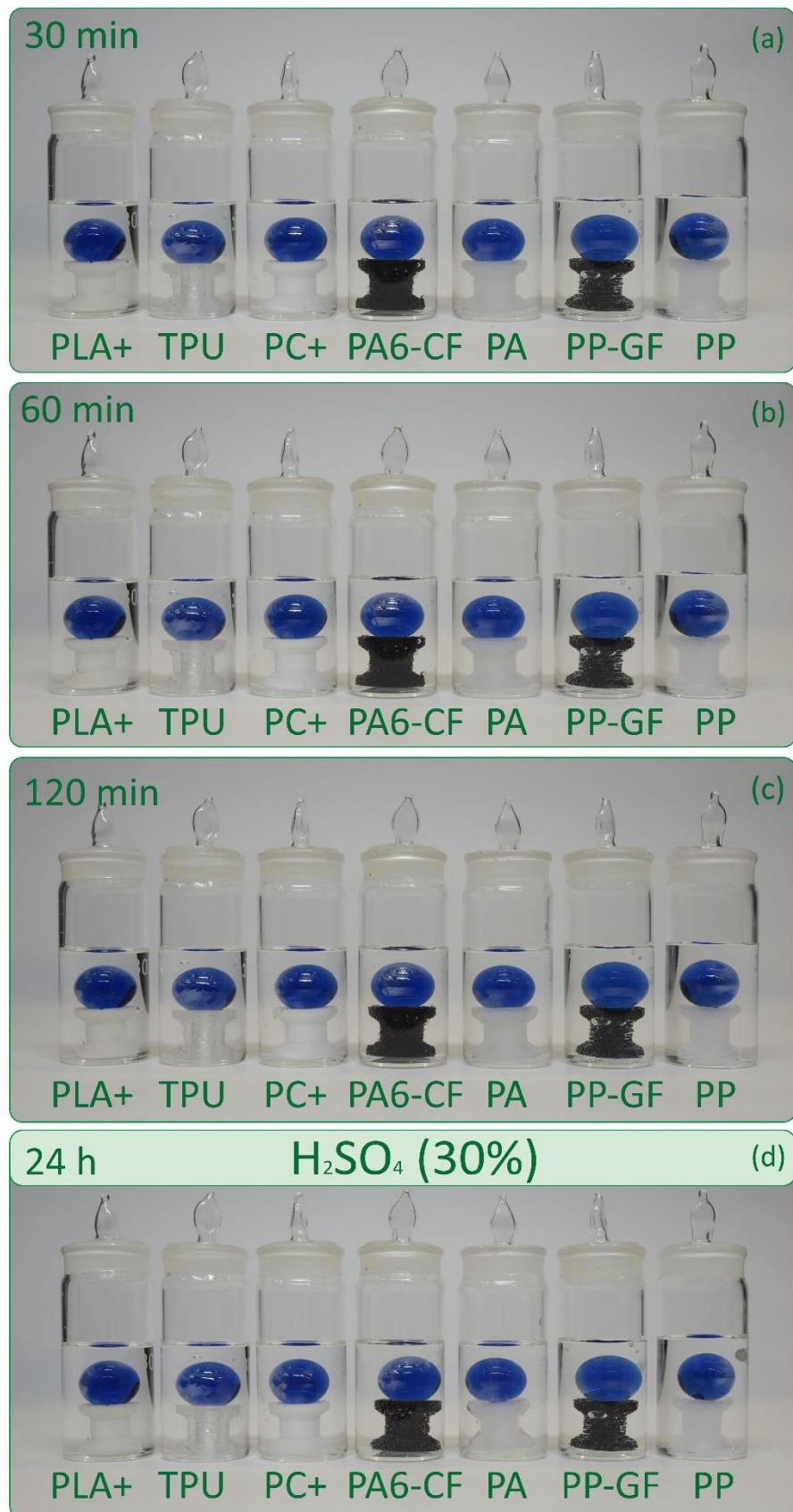
**Figure S8.** Stability test of parts manufactured by the FFF method in sulfuric acid with a concentration of 30% for 24 hours: (a) – result after 30 minutes in a solvent medium; (b) – after 60 min; (c) – after 120 min; (d) – after 2 hours.
