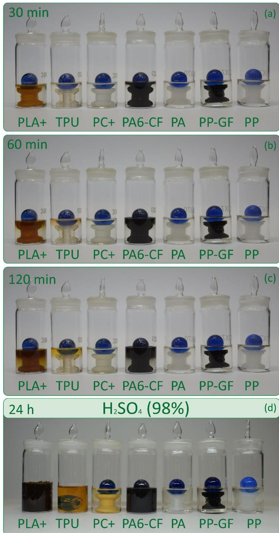
**Figure S9.** Stability test of parts manufactured by the FFF method in sulfuric acid with a concentration of 98% for 24 hours: (a) – result after 30 minutes in a solvent medium; (b) – after 60 min; (c) – after 120 min; (d) – after 2 hours.
