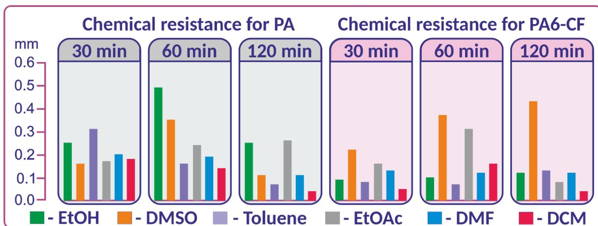
**Figure S23.** Comparative diagram with quantitative calculations of the chemical resistance of 3D printed samples from PA and PA6-CF when exposed to various solvents during different exposure times.
