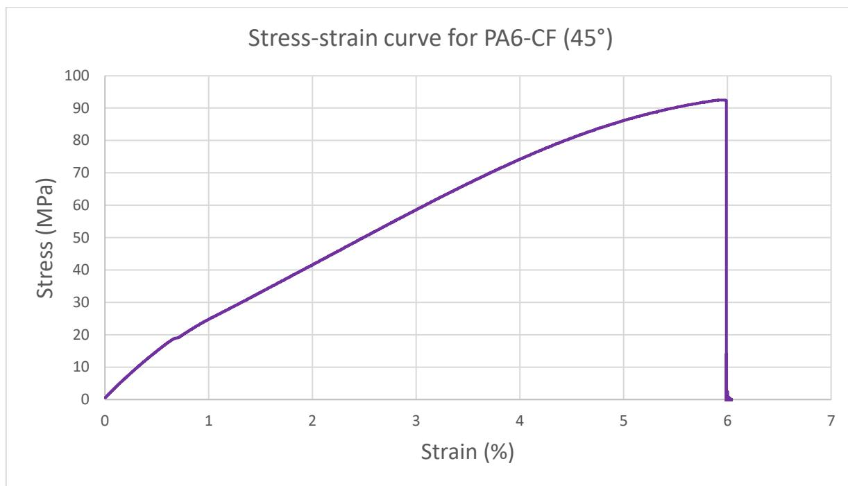
**Figure S43.** Stress-strain graph for a PA6-CF FFF single sample with a print orientation angle equal to 45°.
