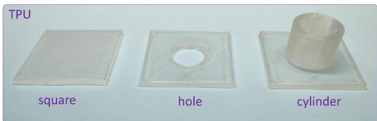
**Figure S55.** TPU parts manufactured by FFF for study of the shrinkage.
