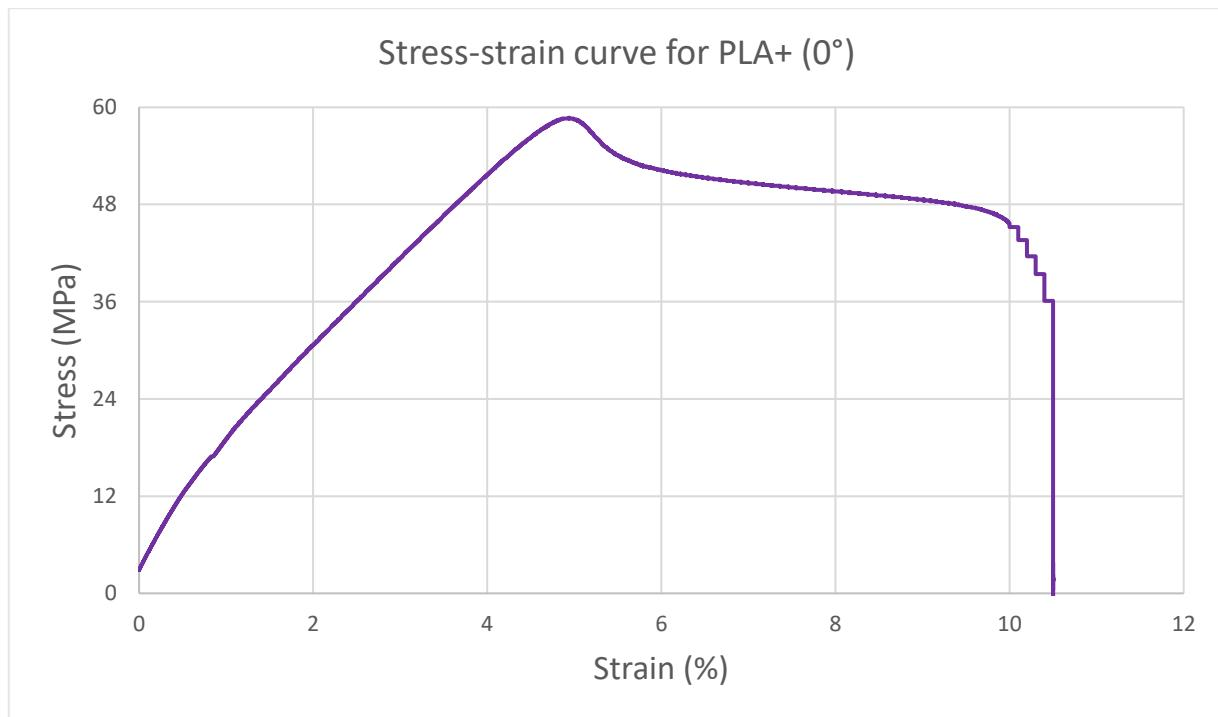
**Figure S33.** Stress-strain graph for a PLA+ FFF single sample with a print orientation angle equal to 0°.
