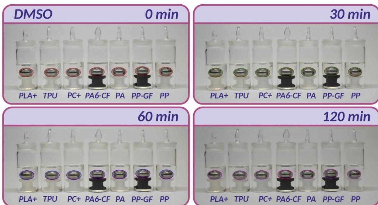
**Figure S17.** Quantitative determination of the chemical resistance of 3D printed samples in dimethyl sulfoxide.
