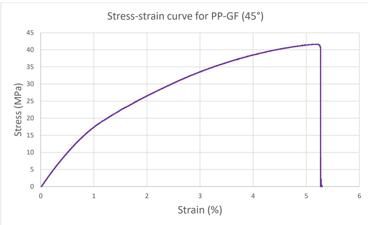
**Figure S45.** Stress-strain graph for a PP-GF FFF single sample with a print orientation angle equal to 45°.
