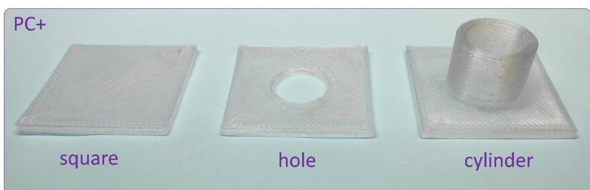
**Figure S56.** PC+ parts manufactured by FFF for study of the shrinkage.
