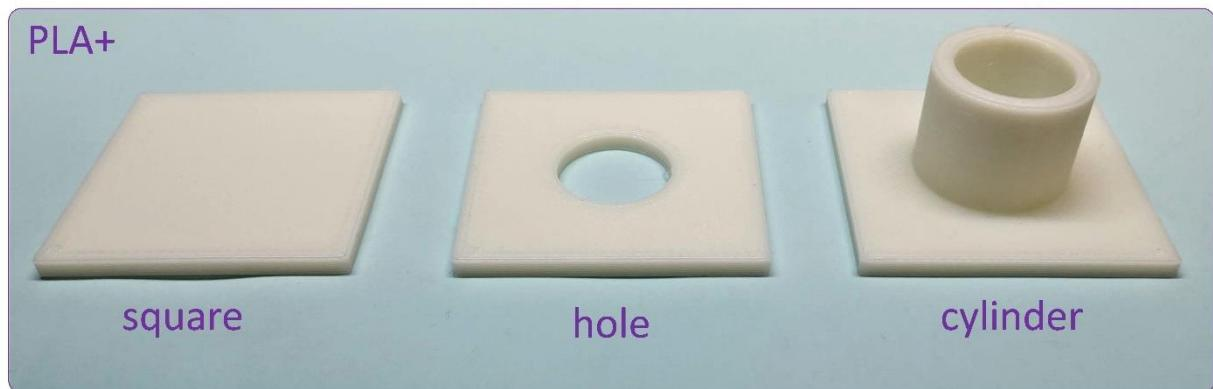
**Figure S54.** PLA+ parts manufactured by FFF for study of the shrinkage.
