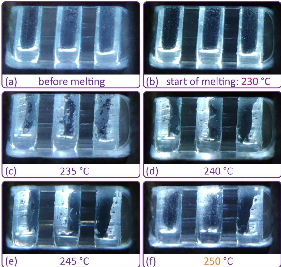
**Figure S25.** Melting point of PA6-CF measured using a melting-point apparatus: (a) – samples before melting; (b) – samples at the moment of the beginning of melting with the corresponding temperature; (c-e) – samples during further melting with the corresponding temperatures; (f) – samples at the moment of melting at the temperature established during the test on the tile.
