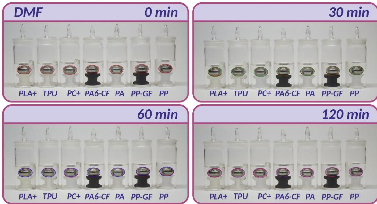
**Figure S14.** Quantitative determination of the chemical resistance of 3D printed samples in dimethylformamide.
