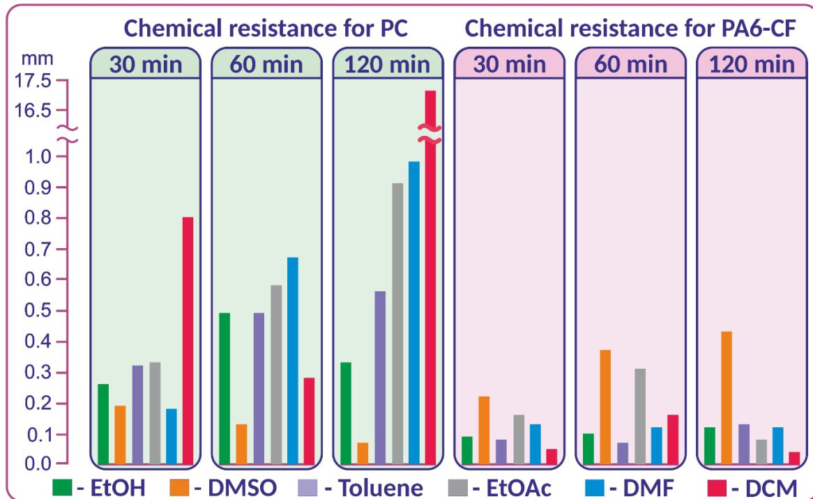
**Figure S22.** Comparative diagram with quantitative calculations of the chemical resistance of 3D printed samples from PC and PA6-CF when exposed to various solvents during different exposure times.
