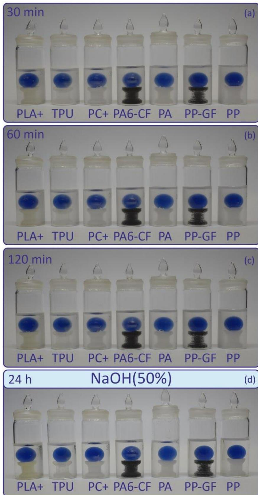
**Figure S12.** Stability test of parts manufactured by the FFF method in sodium hydroxide with a concentration of 50% for 24 hours: (a) – result after 30 minutes in a solvent medium; (b) – after 60 min; (c) – after 120 min; (d) – after 2 hours.
