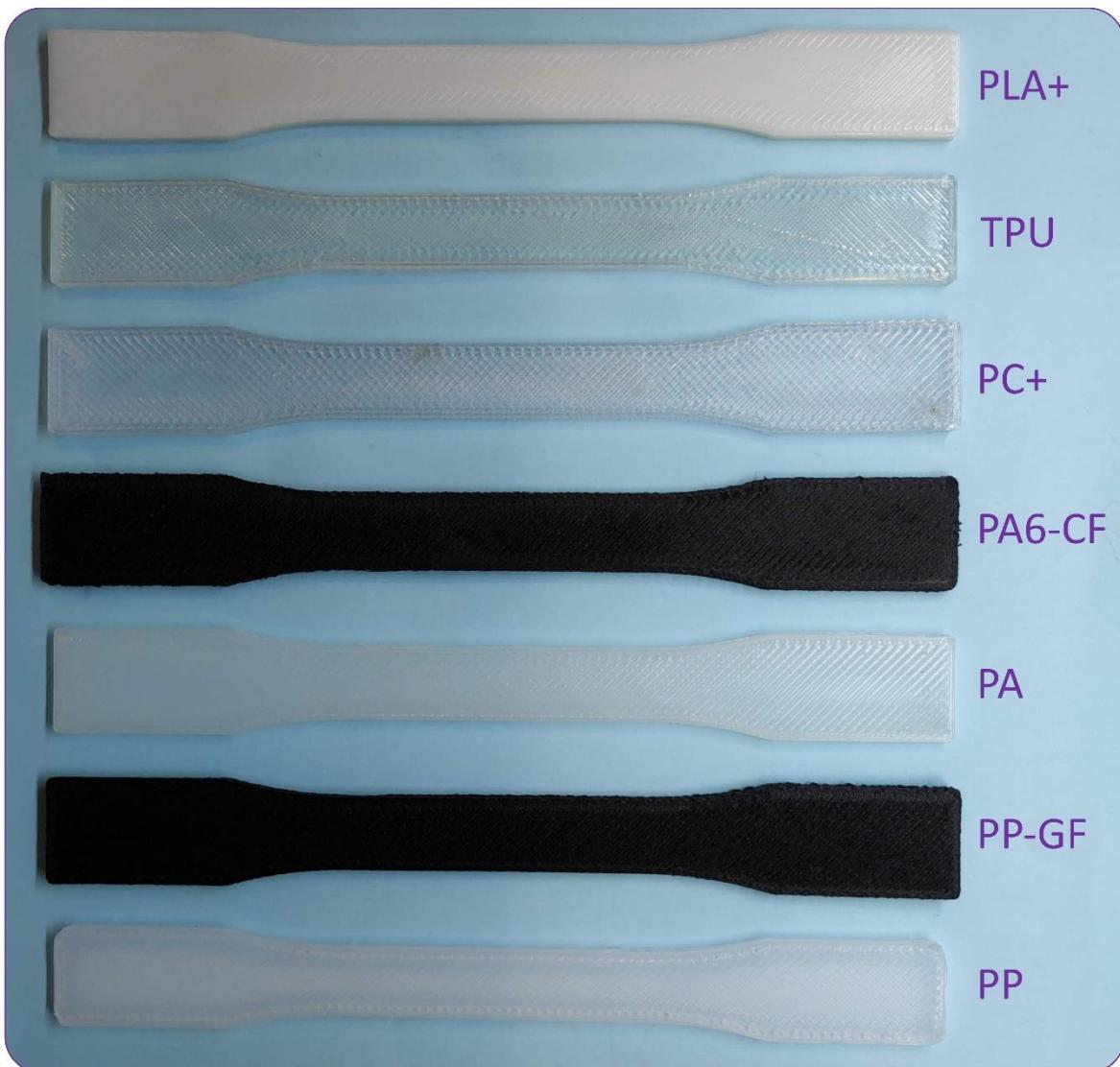
**Figure S31.** FFF samples for tensile testing with infill angle relative to the direction of load application equal to 45°.
