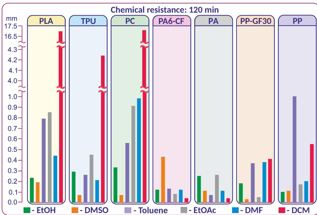
**Figure S21.** Diagram with quantitative calculations of the chemical resistance of 3D printed samples when exposed to various solvents for 120 minutes.
