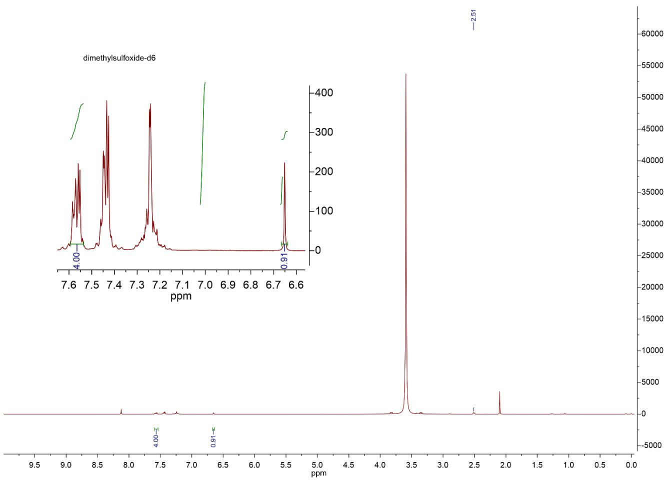
**Figure S72.** <sup>1</sup>H NMR spectrum of the reaction mixture after hydrogenation in the first FFF module of the PA6-CF flow reactor system.
