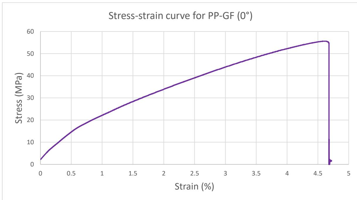
**Figure S38.** Stress-strain graph for a PP-GF FFF single sample with a print orientation angle equal to 0°.
