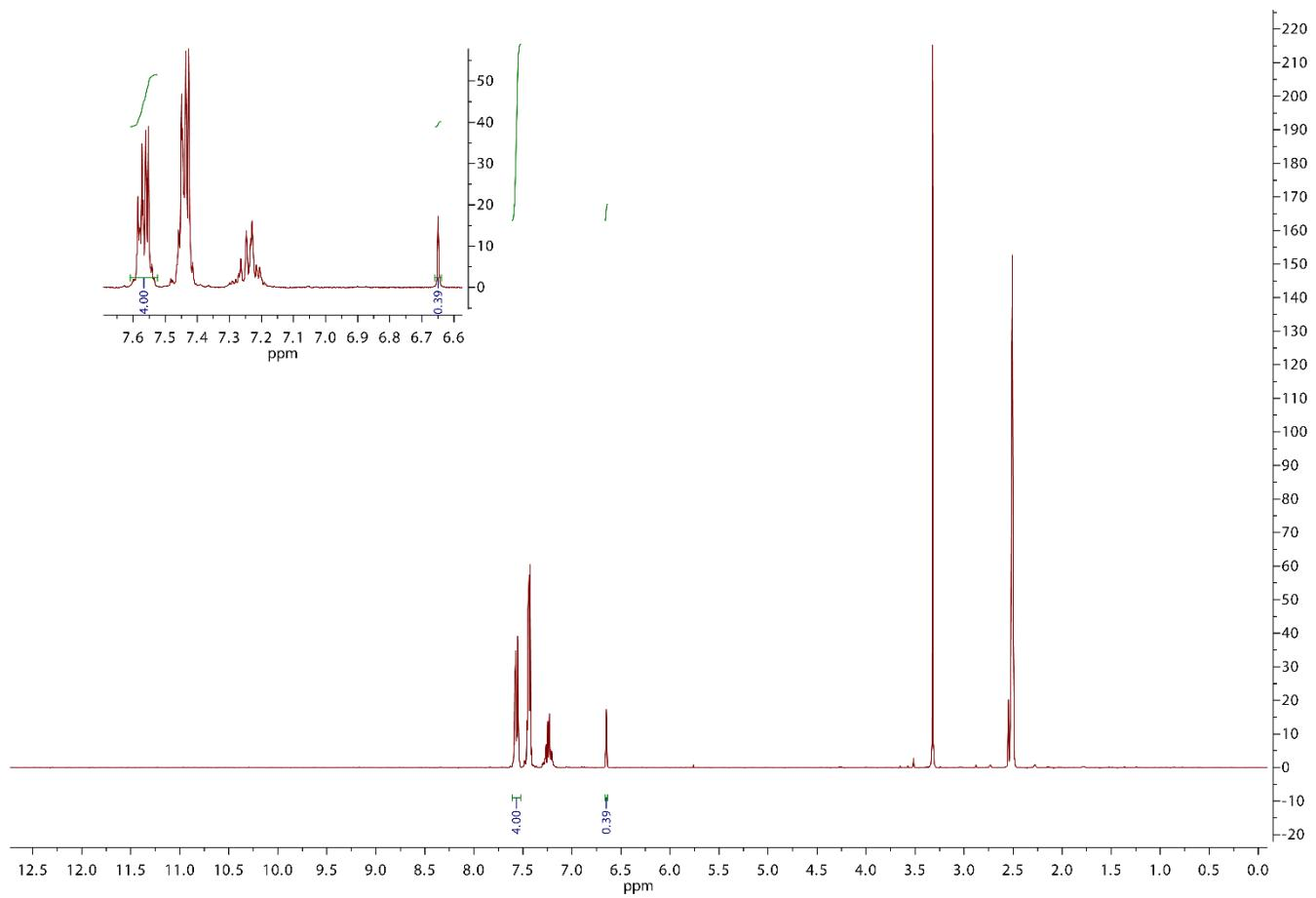
**Figure S67.** <sup>1</sup>H NMR spectrum of the reaction mixture after hydrogenation in FFF batch PA6-CF reactor. The second experimental point for averaging the value of the conversion of diphenylacetylene.
