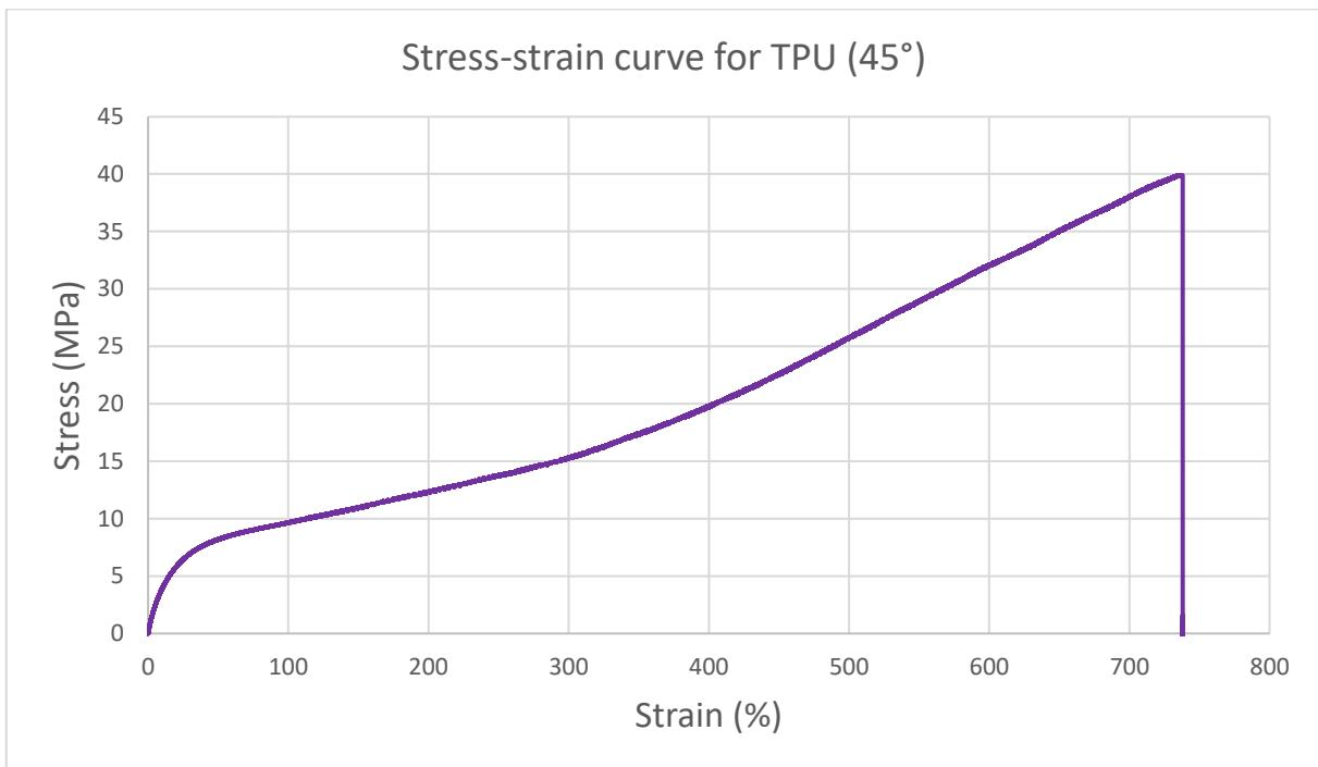
**Figure S41.** Stress-strain graph for a TPU FFF single sample with a print orientation angle equal to 45°.
