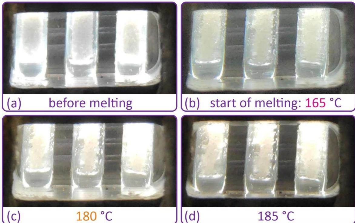
**Figure S27.** Melting temperature of PLA+ measured using a melting-point apparatus: (a) – samples before melting; (b) – samples at the moment of the beginning of melting with the corresponding temperature; (c) – samples at the moment of melting at the temperature established during the test on the tile; (d) – samples during further melting with the corresponding temperature.
