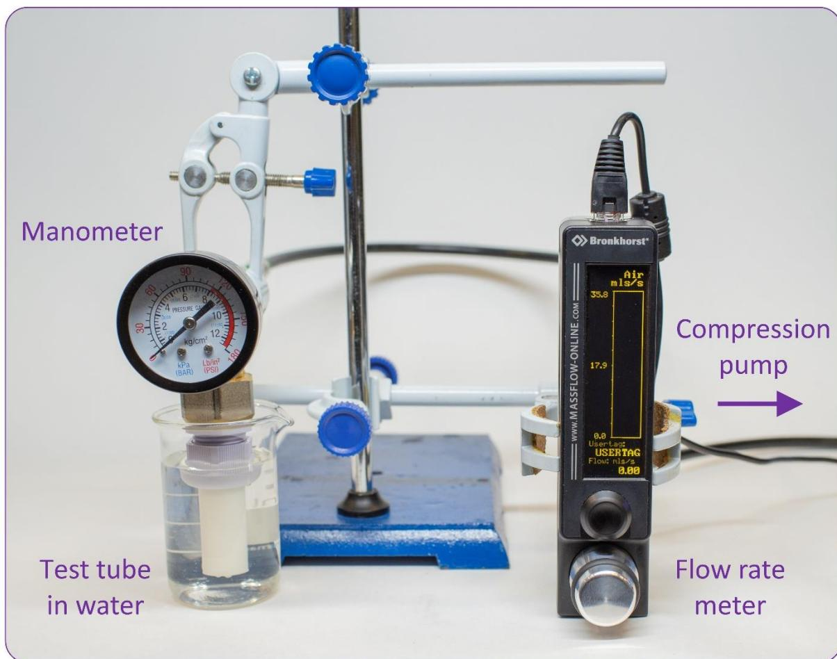
**Figure S47.** Installation for determining the microporosity of products.
