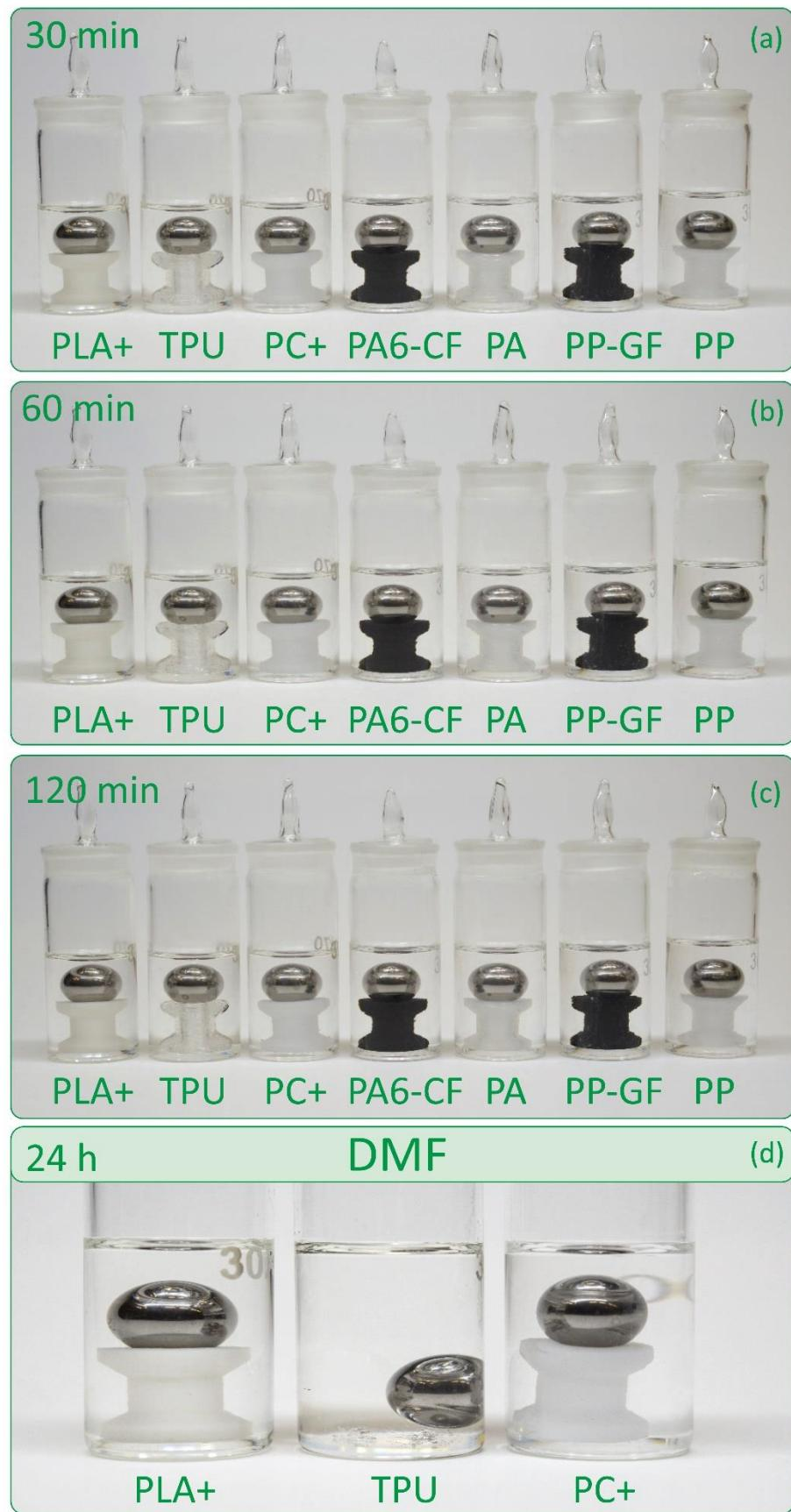
**Figure S5.** Stability test of parts manufactured by the FFF method in a dimethylformamide medium for 24 hours: (a) after 30 minutes in a solvent medium; (b) after 60 min; (c) after 120 min; (d) after 2 hours.
