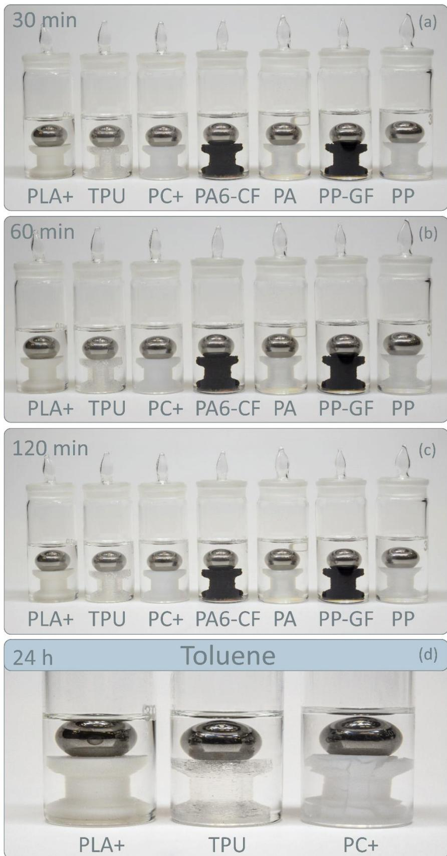
**Figure S3.** Stability test of parts manufactured by the FFF method in toluene for 24 hours: (a) – result after 30 minutes in a solvent medium; (b) – after 60 min; (c) – after 120 min; (d) – after 2 hours.
