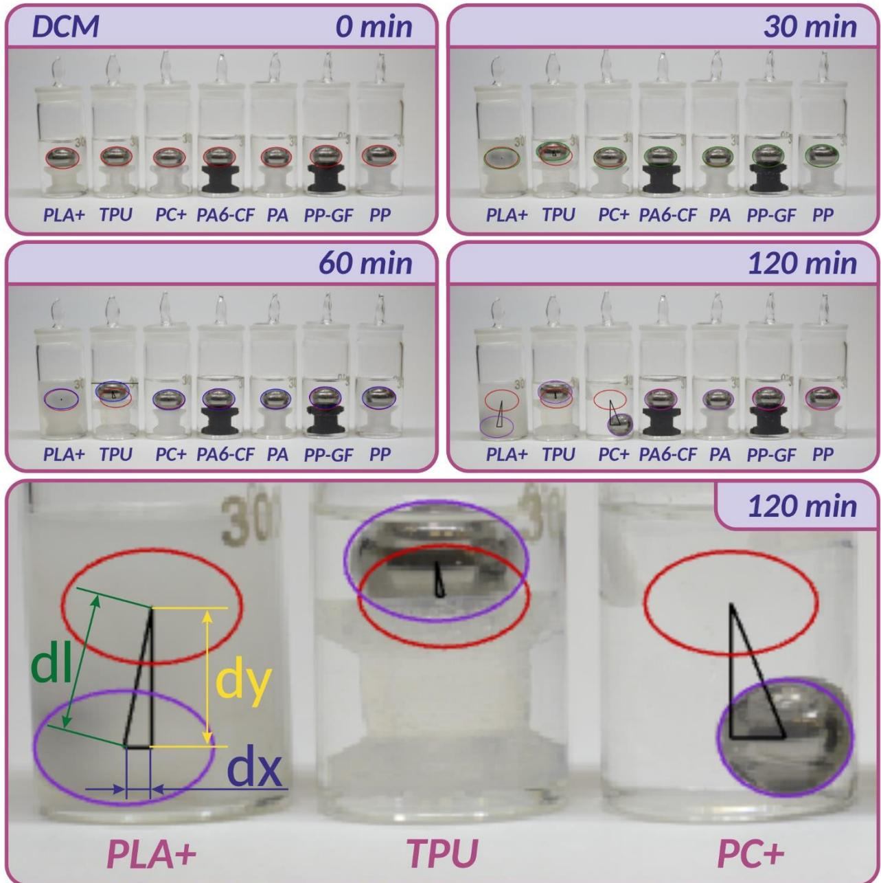
**Figure S13.** Quantitative determination of the chemical resistance of 3D printed samples in methylene chloride.
