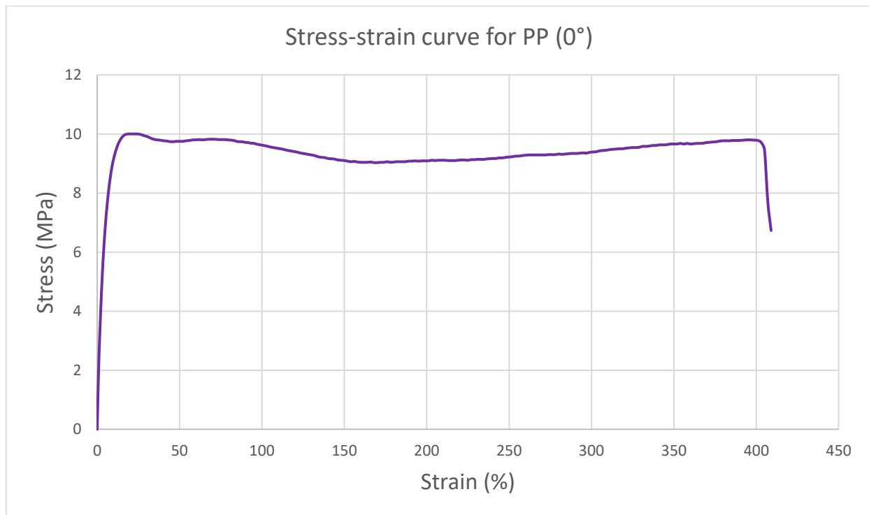
**Figure S39.** Stress-strain graph for a PP FFF single sample with a print orientation angle equal to 0°.
