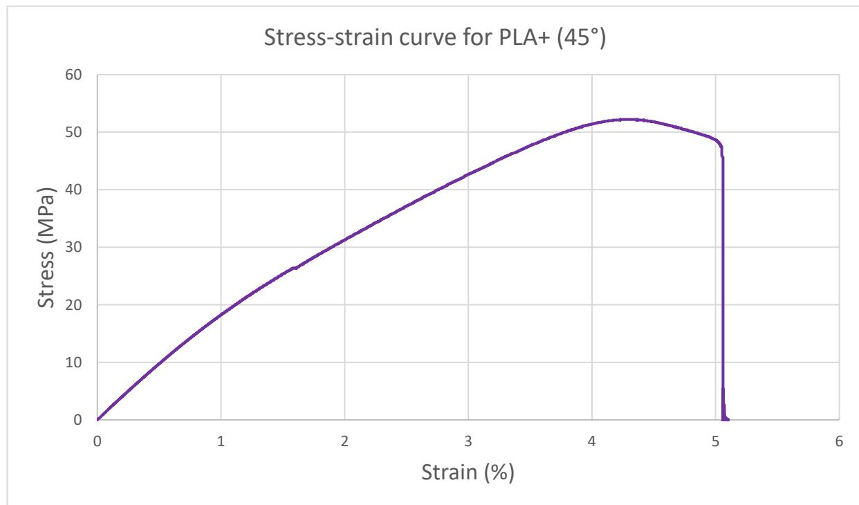
**Figure S40.** Stress-strain graph for a PLA+ FFF single sample with a print orientation angle equal to 45°.
