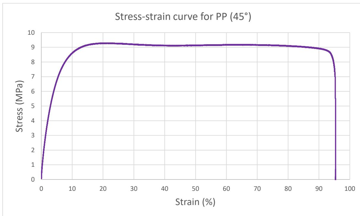
**Figure S46.** Stress-strain graph for a PP FFF single sample with a print orientation angle equal to 45°.
