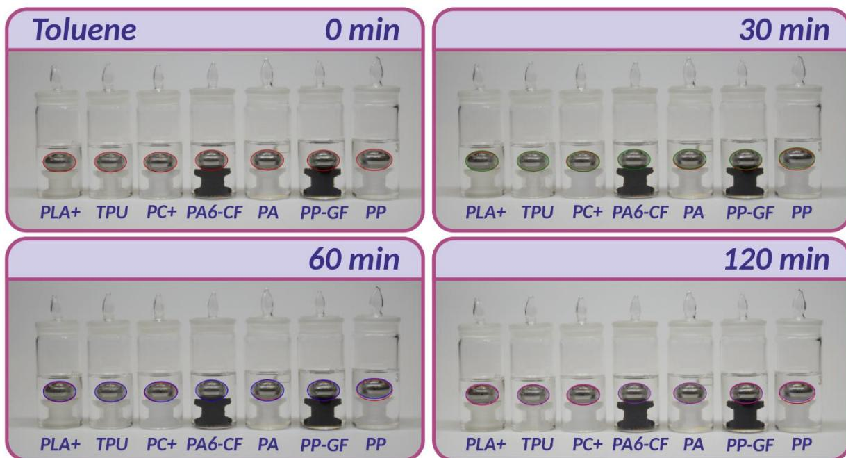
**Figure S16.** Quantitative determination of the chemical resistance of 3D printed samples in toluene.
