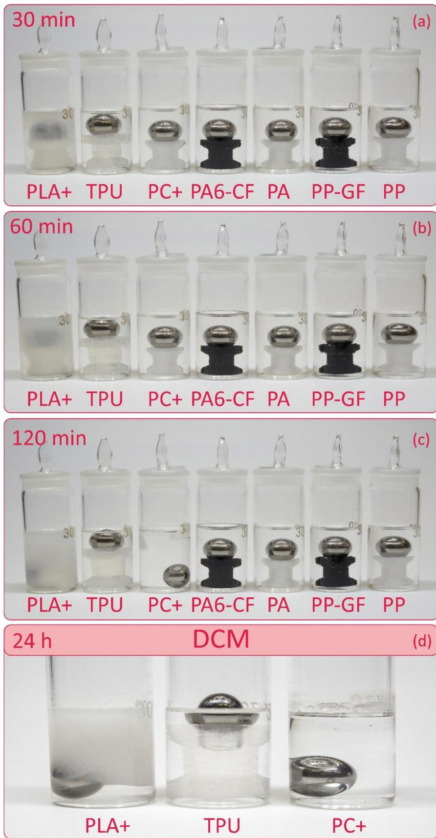
**Figure S6.** Stability test of parts manufactured by the FFF method in methylene chloride for 24 hours: (a) – result after 30 minutes in a solvent medium; (b) – after 60 min; (c) – after 120 min; (d) – after 2 hours.
