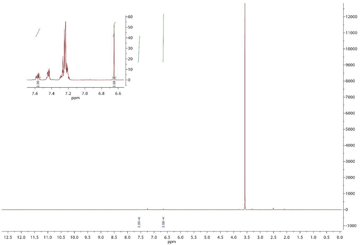
**Figure S64.** <sup>1</sup>H NMR spectrum of the reaction mixture after hydrogenation in FFF batch PA reactor. The fourth experimental point for averaging the value of the conversion of diphenylacetylene.
