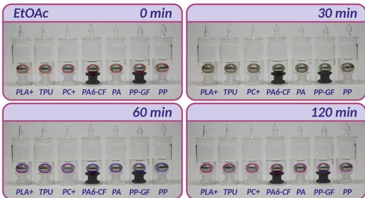
**Figure S15.** Quantitative determination of the chemical resistance of 3D printed samples in ethyl acetate.
