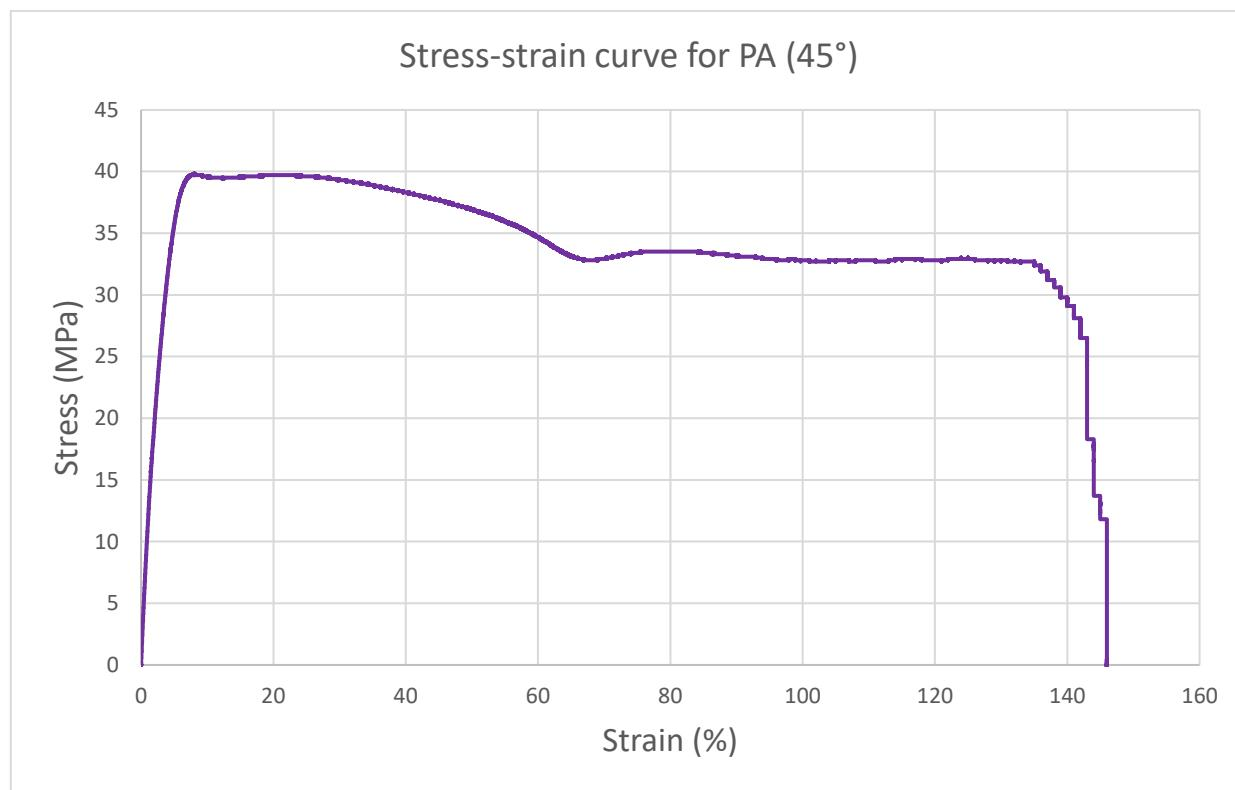
**Figure S44.** Stress-strain graph for a PA FFF single sample with a print orientation angle equal to 45°.
