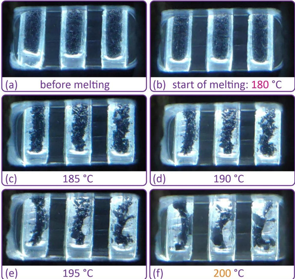
**Figure S29.** Melting point of PP-GF measured using a melting-point apparatus: (a) – samples before melting; (b) – samples at the moment of the beginning of melting with the corresponding temperature; (c-e) – samples during further melting with the corresponding temperatures; (f) – samples at the time of melting at the temperature established during the test on the tile.
