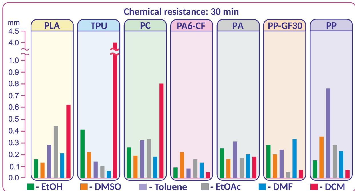
**Figure S19.** Diagram with quantitative calculations of the chemical resistance of 3D printed samples when exposed to various solvents for 30 minutes.
