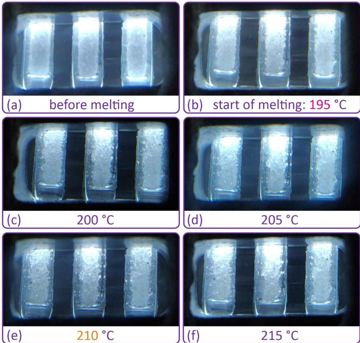
**Figure S26.** Melting point of PC+ measured using a melting-point apparatus: (a) – samples before melting; (b) – samples at the moment of the beginning of melting with the corresponding temperature; (c), (d) – samples during further melting with the corresponding temperatures; (e) – samples at the time of melting at the temperature established during the test on the tile; (f) – samples during further melting with the corresponding temperature.
