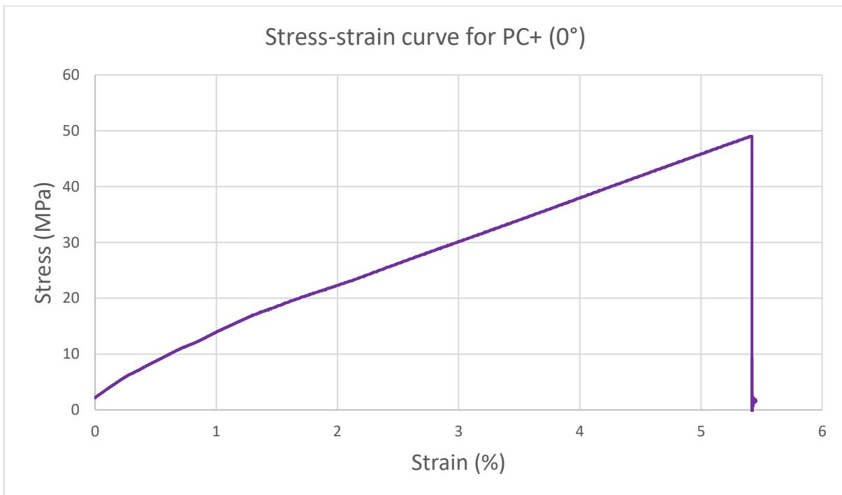
**Figure S35.** Stress-strain graph for a PC+ FFF single sample with a print orientation angle equal to 0°.
