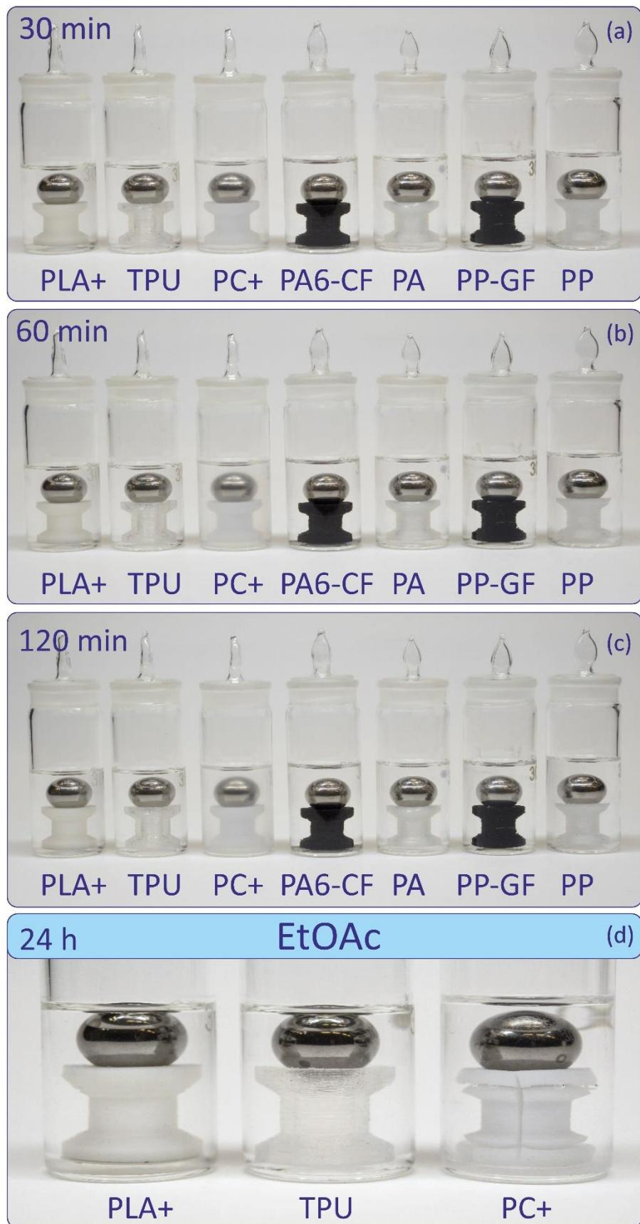
**Figure S4.** Stability test of parts manufactured by the FFF method in ethyl acetate medium for 24 hours: (a) – result after 30 minutes in a solvent medium; (b) – after 60 min; (c) – after 120 min; (d) – after 2 hours.
