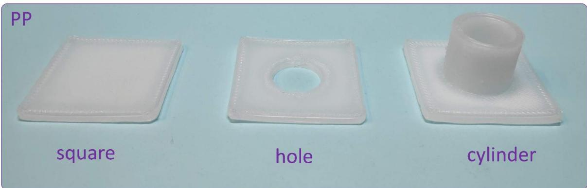
**Figure S60.** PP parts manufactured by FFF for study of the shrinkage.
