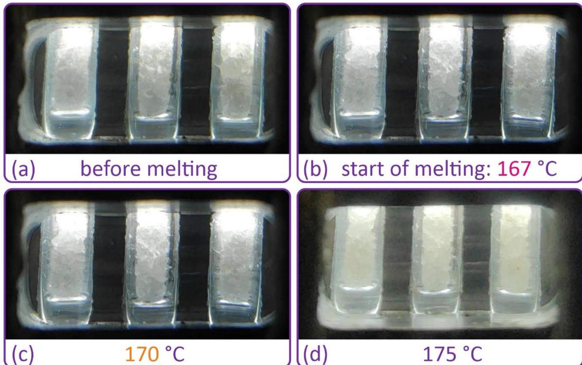
**Figure S30.** Melting point of TPU measured using a melting-point apparatus: (a) – samples before melting; (b) – samples at the moment of the beginning of melting with the corresponding temperature; (c) – samples at the moment of melting at the temperature established during the test on the tile; (d) – samples during further melting with the corresponding temperature.
