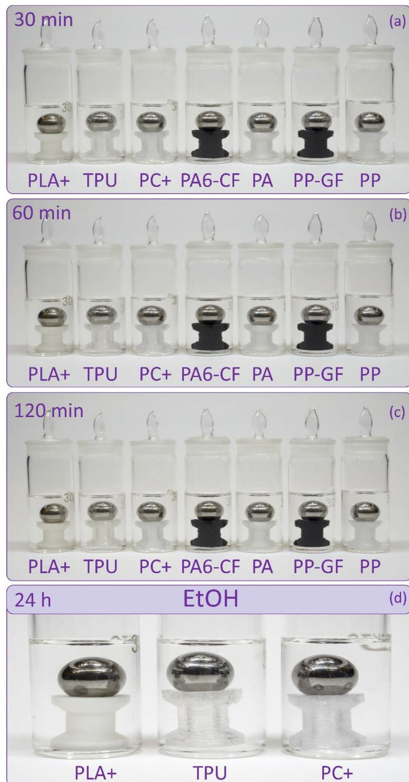
**Figure S1.** Stability test of parts manufactured by the FFF method in ethanol medium for 24 hours: (a) – result after 30 min in a solvent environment; (b) – after 60 min; (c) – after 120 min; (d) – after 2 hours.
