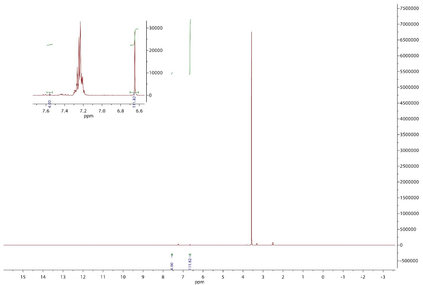
**Figure S61.** <sup>1</sup>H NMR spectrum of the reaction mixture after hydrogenation in FFF batch PA reactor. The first experimental point for averaging the value of the conversion of diphenylacetylene.
