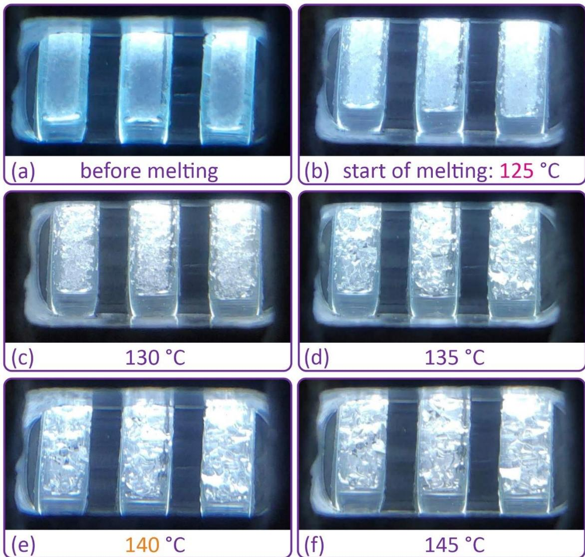
**Figure S28.** Melting temperature of PP measured using a melting-point apparatus: (a) – samples before melting; (b) – samples at the moment of the beginning of melting with the corresponding temperature; (c), (d) – samples during further melting with the corresponding temperatures; (e) – samples at the time of melting at the temperature established during the test on the tile; (f) – samples during further melting with the corresponding temperature.
