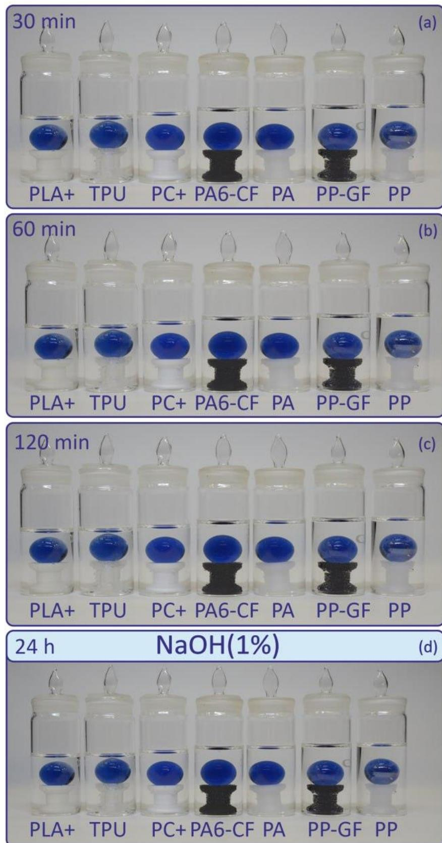
**Figure S10.** Stability test of parts manufactured by the FFF method in sodium hydroxide with a concentration of 1% for 24 hours: (a) – result after 30 minutes in a solvent medium; (b) – after 60 min; (c) – after 120 min; (d) – after 2 hours.
