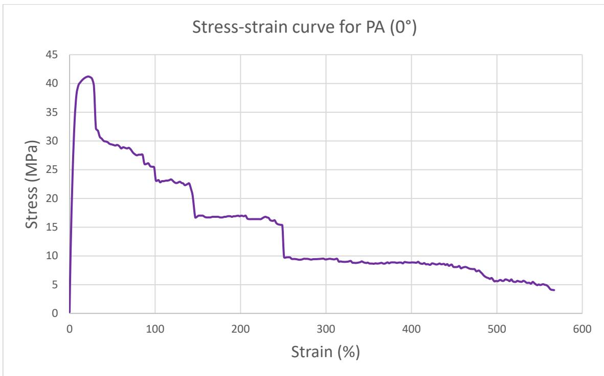
**Figure S37.** Stress-strain graph for a PA FFF single sample with a print orientation angle equal to 0°.
