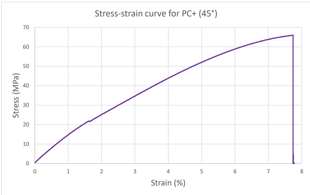
**Figure S42.** Stress-strain graph for a PC+ FFF single sample with a print orientation angle equal to 45°.
