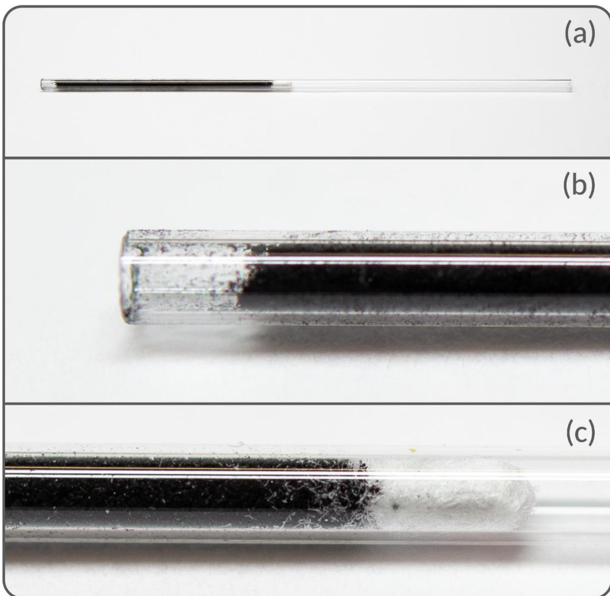
**Figure S71.** Catalytic tube with filter, filled Pd/C (10%) and K<sub>2</sub>CO<sub>3</sub>.
