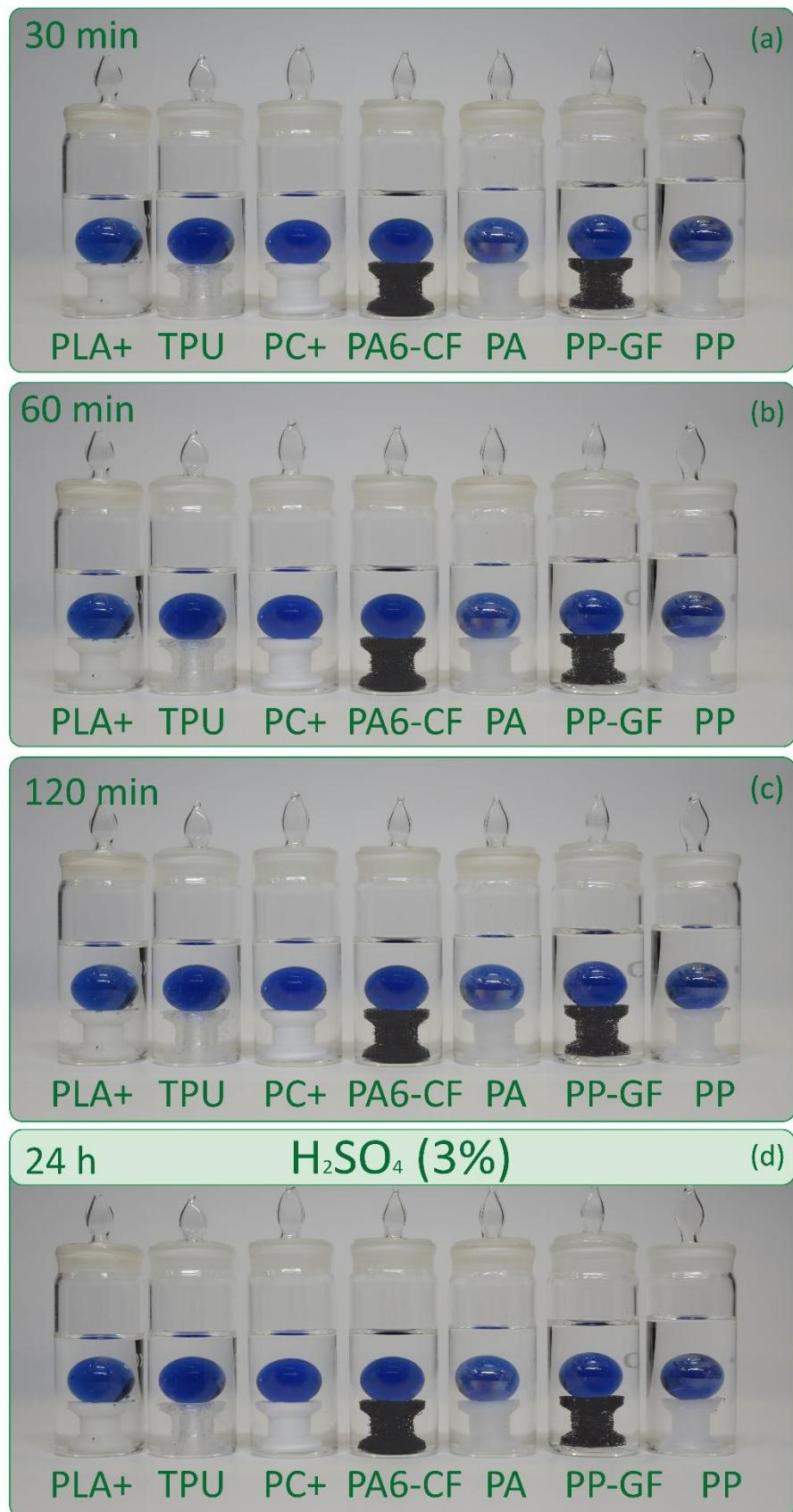
**Figure S7.** Stability test of parts manufactured by the FFF method in sulfuric acid with a concentration of 3% for 24 hours: (a) – result after 30 minutes in a solvent medium; (b) – after 60 min; (c) – after 120 min; (d) – after 2 hours.
