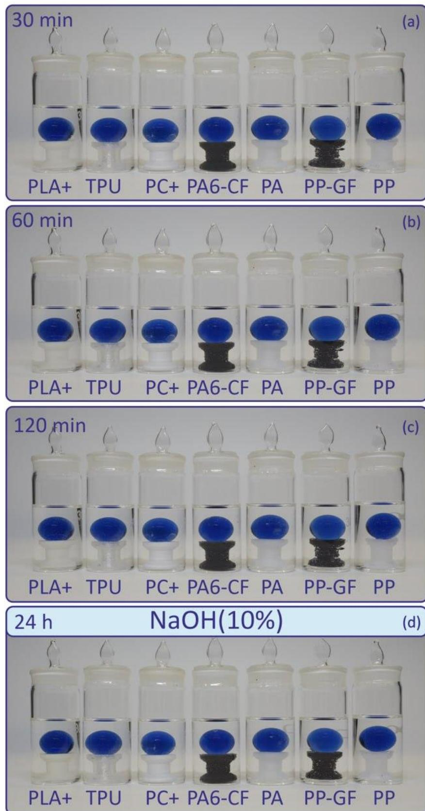
**Figure S11.** Stability test of parts manufactured by the FFF method in sodium hydroxide with a concentration of 10% for 24 hours: (a) – result after 30 minutes in a solvent medium; (b) – after 60 min; (c) – after 120 min; (d) – after 2 hours.
