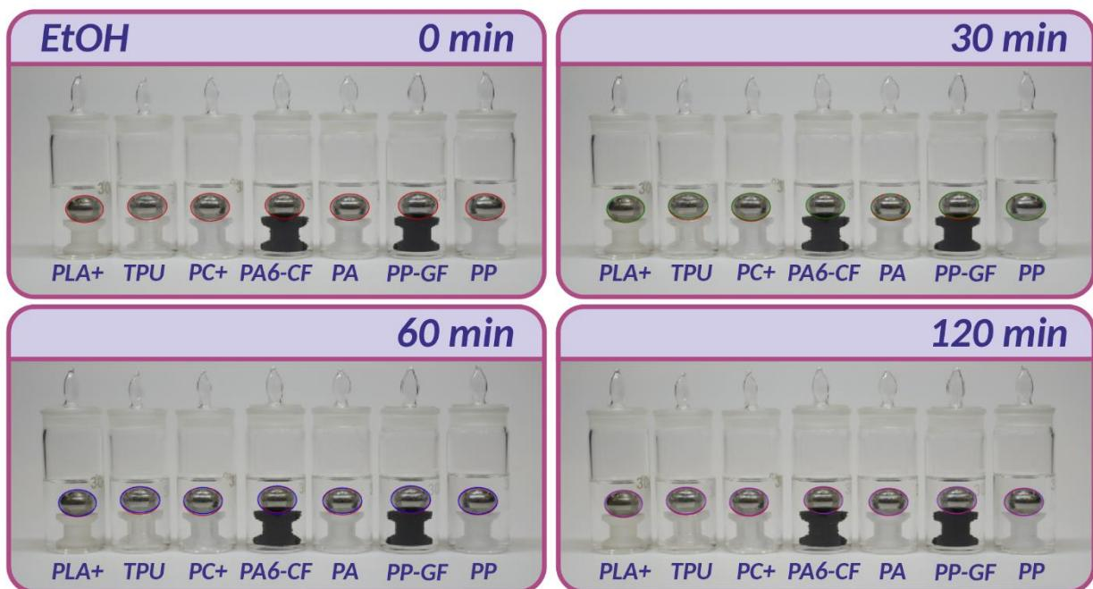
**Figure S18.** Quantitative determination of the chemical resistance of 3D printed samples in ethanol.
