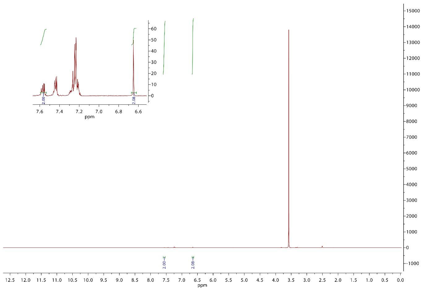
**Figure S65.** <sup>1</sup>H NMR spectrum of the reaction mixture after hydrogenation in FFF batch PA reactor. The fifth experimental point for averaging the value of the conversion of diphenylacetylene.
