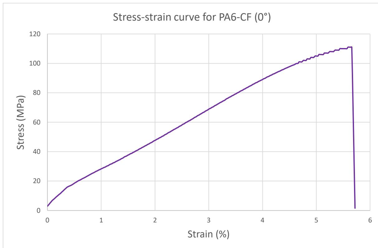
**Figure S36.** Stress-strain graph for a PA6-CF FFF single sample with a print orientation angle equal to 0°.
