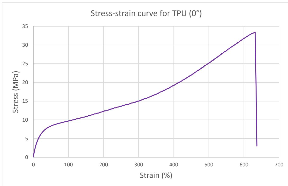
**Figure S34.** Stress-strain graph for a TPU FFF single sample with a print orientation angle equal to 0°.
