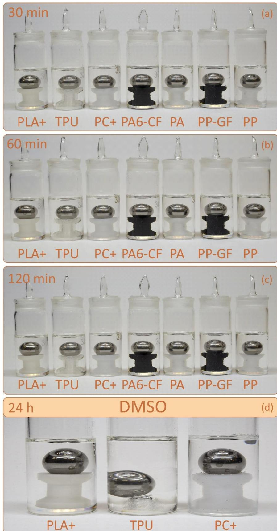
**Figure S2.** Stability test of parts manufactured by the FFF method in dimethyl sulfoxide for 24 hours: (a) – result after 30 minutes in a solvent medium; (b) – after 60 min; (c) – after 120 min; (d) – after 2 hours.
