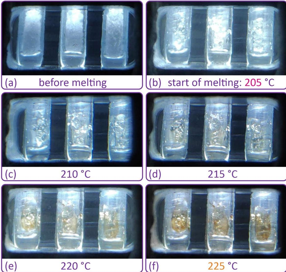
**Figure S24.** Melting point of PA measured using a melting-point apparatus: (a) – samples before melting; (b) – samples at the moment of the beginning of melting with the corresponding temperature; (c-e) – samples during further melting with the corresponding temperatures; (f) – samples at the time of melting at the temperature established during the test on the tile.
