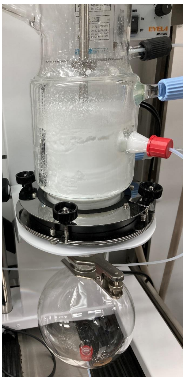
Figure S9: A picture of the thin layer evaporator that have crystallized peptide 4 in the chamber
