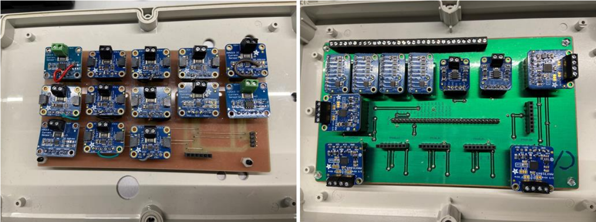
Figure S8 Left: printed circuit board and INA219 breakout boards for calibration of the PEs and measurement of electrical current during isothermal operation mode. Right: printed circuit board and respective breakout boards for calorimetric measurements
