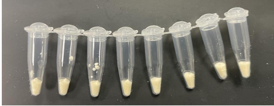
Figure S11. A picture showing lyophilized PolyPt in PCR tubes (ca. 300 \mu\text{g} per tube).
