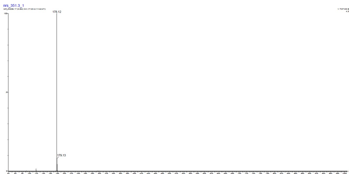
Figure S21. Mass spectrum of Ald under electrospray ionization in positive ion mode.
