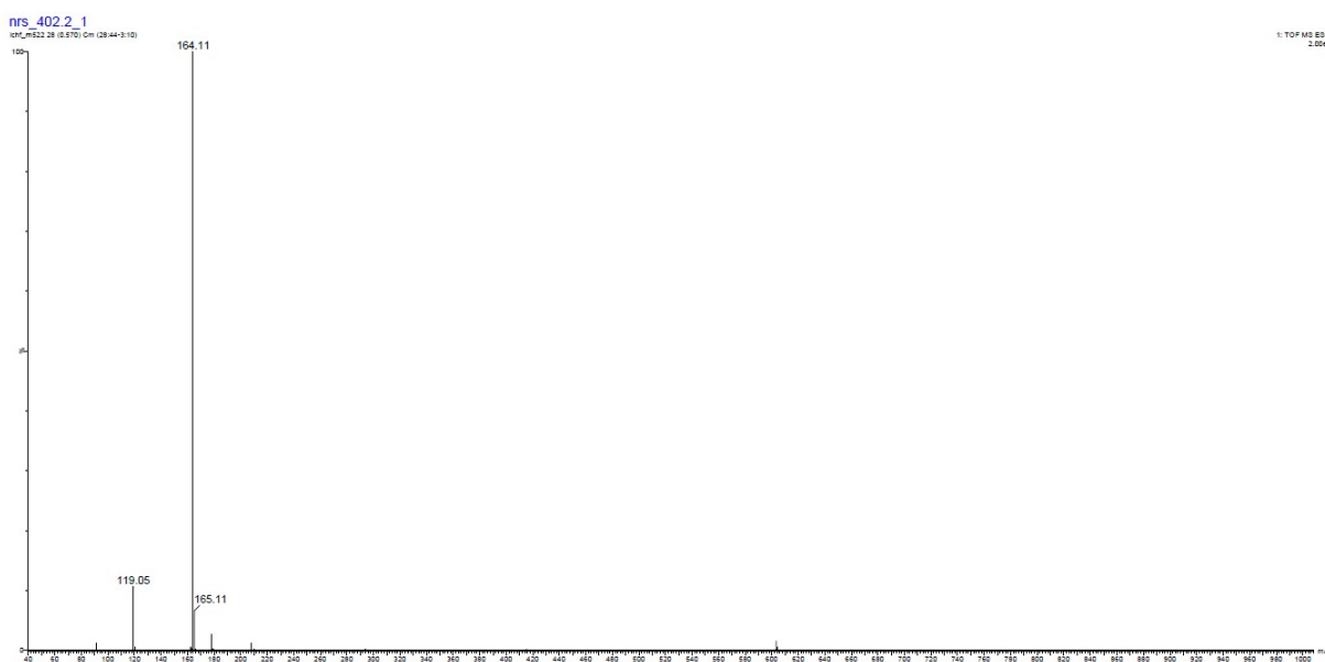
Figure S19. Mass spectrum of 6 under electrospray ionization in positive ion mode.
