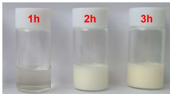
Figure S6. Photograph of TS-1-TBOT (also named as TS-1-TBOT-10) samples crystallized at 170 °C for different times.
