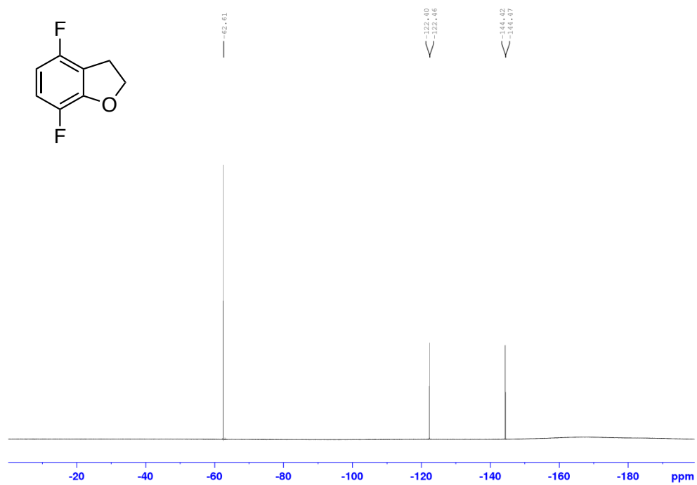
19 F NMR spectrum of 30 (377 MHz, CDCl 3 , PhCF 3 internal standard set at -62.61 ppm)
