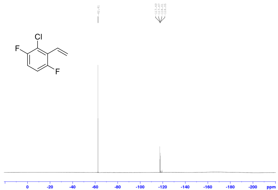
^{19}\text{F} NMR spectrum of 2-chloro-3,6-difluorostyrene (377 MHz, \text{CDCl}_3 , \text{PhCF}_3 internal standard set at -62.61 ppm)
