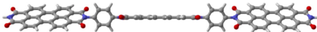
Figure S85. DFT-calculated structure of a portion of PTCDA-pPDA , suggesting that the polymer is not fully conjugated.
