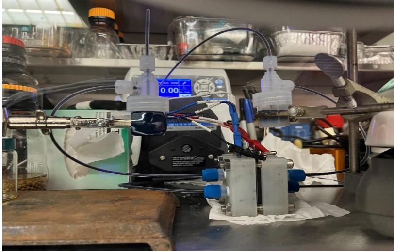
Figure SI-2: Picture of flow cell during operation.
