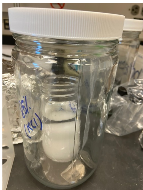
Figure S26. Artificial 85% humidity chamber.
