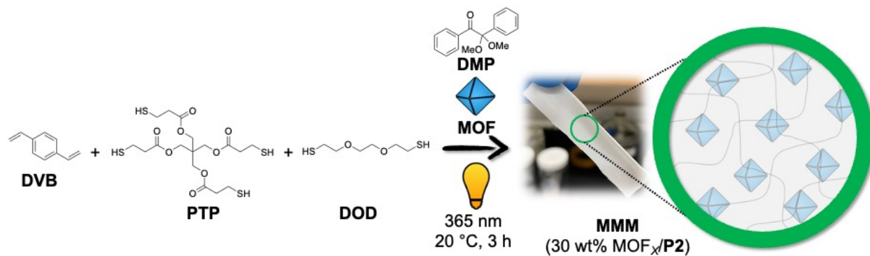
Figure S5. Scheme for synthesizing P2 -based (control, not self-healing) MMMs with 30 wt% MOF-loading using thiol-ene 'photo-click' polymerization.
