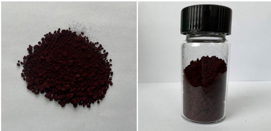
**Figure S2.** Photos of PSQ obtained from a one-pot polymerization process (the mass of PSQ is ca. 4 g, yield 92%).
