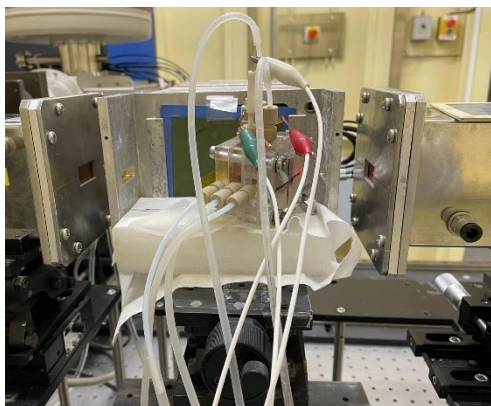
Fig. S16. Operando electrochemical cell for XAS test.
