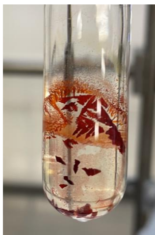
S-Figure 1: Crystals of 1 isolated at low-temperatures via crystallization from 1,2-DFB/ n -heptane.
