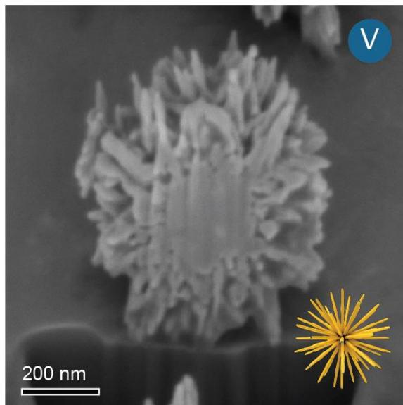
**Figure S 4** SEM image of FIB-milled cross-section of an urchin (Figure 1 V).
