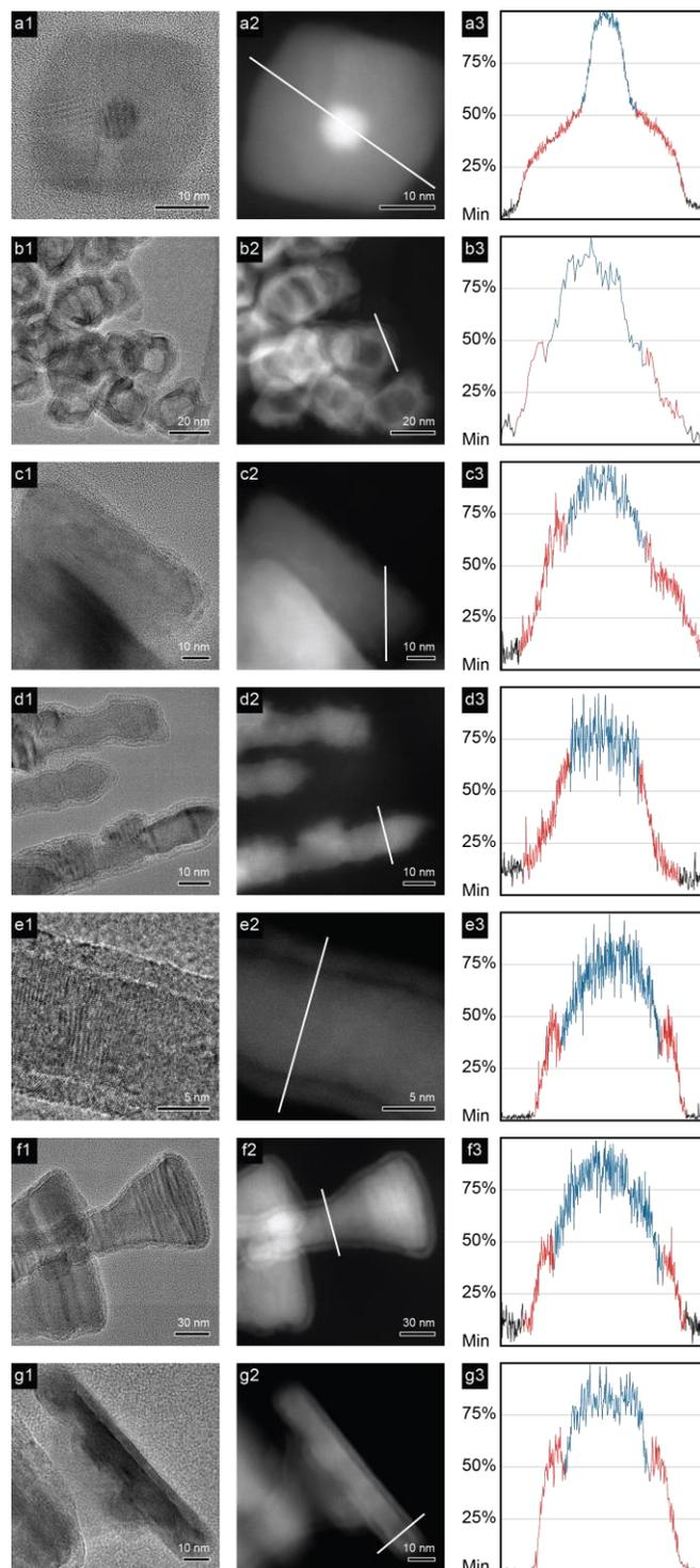
**Figure S 3** TEM images (column 1), STEM images (column 2), and the corresponding contrast profiles (column 3) of various Ni@Ni<sub>3</sub>C nanostructures.
