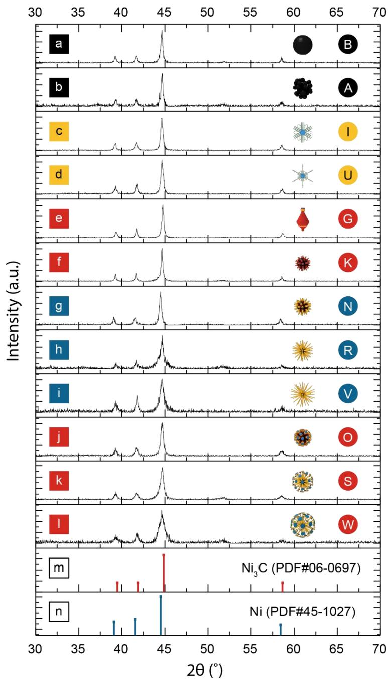
**Figure S 2** XRD patterns of selected NBCs. (a) Dots; (b) clusters; (c, d) dendrites; (e, f) polyhedra and its aggregates; (g, h, i) urchins; (j, k, l) dandelions; (m)  $\text{Ni}_3\text{C}$  standard (JCPDS PDF #06-0697); (n) Ni standard (JCPDS PDF #45-1027). (The letter on the left indicates the order in this figure; the circled letter on the right indicates the NBC's serial number in Figure 1).
