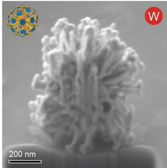
**Figure S 5** SEM image of FIB-milled cross-section of a dandelion (Figure 1 W).
