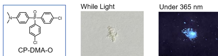
Fig. S5 Photographs of CP-DMA-O taken under while light and UV lamp ( 365\text{ nm} , 150\text{ mW}\cdot\text{cm}^{-2} ).
